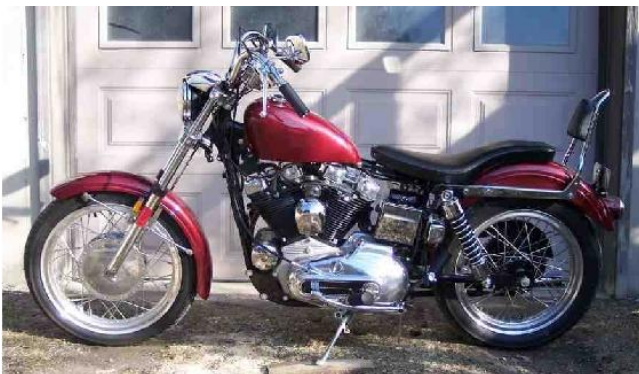
The 1971 XLCH has the electric starter hump, but they don't install it. The small battery is a giveaway this is kickstart.
