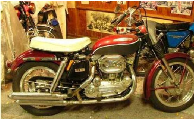
This 1969 XLH Iron Sportster features the interconnected dual exhaust with the long mufflers.
