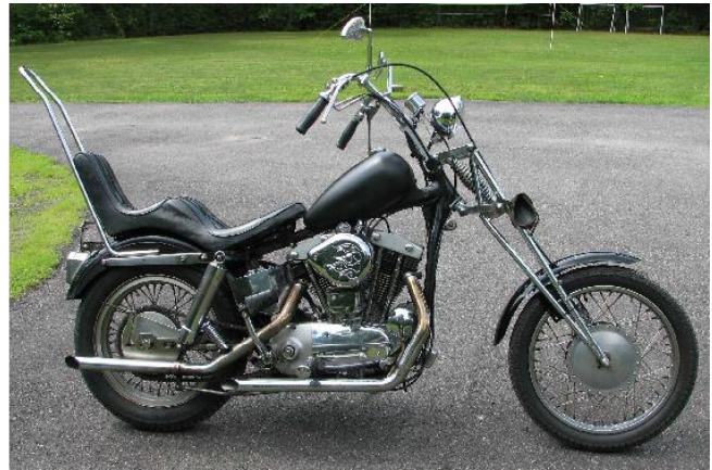
A girder front end is clean and light on this 1960 chop. There is no battery to worry about on a magneto bike. With a sprung rear end, for those with back problems.
