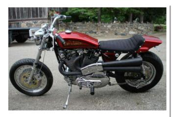
The front suspension consists of a Ceriani roadrace fork that has been show chromed. The brake discs (11 and 12") are Meehanite (produced by Kosman), with the calipers coming from Performance Machine (four piston fronts, 2 piston rear).
