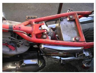
Here is the monoshock setup Kenny Puccio welded up. All he did was cut the battery tray out of the standard 1979-80 oil tank so the shock can pass through. I don't think he even had to lengthen the swingarm.
