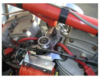
The engine mount ties in with the tank mount, something I am not too fond of. The mount broke, probably due to my carrying groceries on top of the tank. That hack weld job is mine, not Kenny's. I have an XLCR tank I am going to put on. I detest fiberglass tanks. They are known to explode when you drop the bike, and this one sprang a leak and caused years of mystery as I tried to get another custom fiberglass tank made, with all the attendant petcock and fuel delivery problems.
