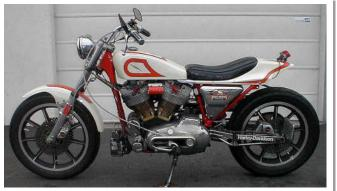
The tail light was mounted under the fender, but the rear tire would hit it on full jounce and knock the lens off. I just flipped up to the top and mounted it in the same holes.
