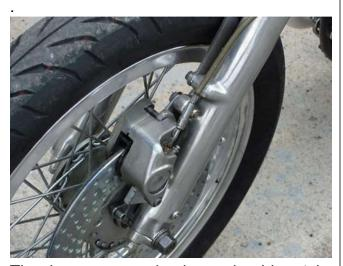
The rims are new aluminum shoulder style with polished spokes to reflect the Harley racing heritage. The front tire is 100/90/19" and the rear is 110/90/18".
