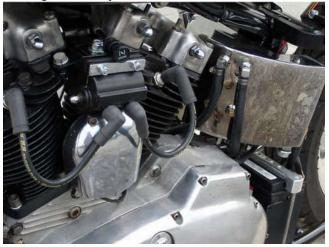
There was a problem was with the RPM in relationship to road speed. At 60 to 70 mph the engine felt like it needed another gear. This made the engine work at a higher temperature than I would like it to be, plus it caused internal problems. To solve this we went from a factory 21 to a 23 tooth front sprocket. A new chain was used.
