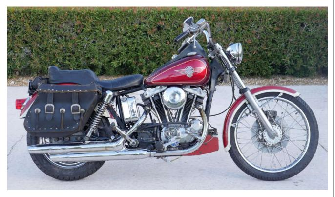
She started life a stock XLCH kickstartonly bike. This last rebuild I put on a set of big bike tanks, fenders and saddlebags. I had previously had the electric starter pocket cut off and adapted an Evo-era primary cover. I also put in the pre-1970 dry clutch that I run wet with Barnett Kevlar plates. I fabricated a clutch mechanism and a kickstart support bracket. I removed the peg mounts from the engine and put them on the frame like 1976 and earlier bikes.
