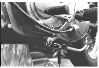
I welded peg mounts on the frame to use the early model footpegs. I don't like pegs mounted on the engine.
