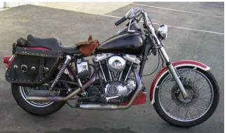
Before the Softtail tanks, I had a set of 5-gallon flat-side tanks for range.
