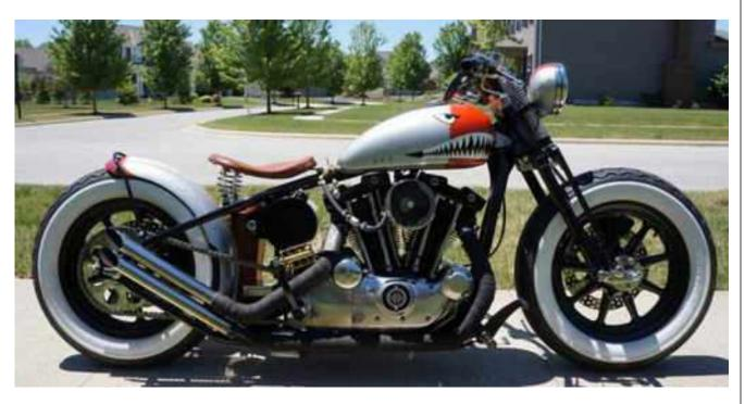
You will be stopped when gassing up for pictures, etc. There is nothing like kick-starting it at your local bike night. I even won a trophy with it. This bike has a weld-on hardtail and uses a DNA Springer front fork (4.5 inches under stock) to both lower and stretch the bike 4 inches respectively.
