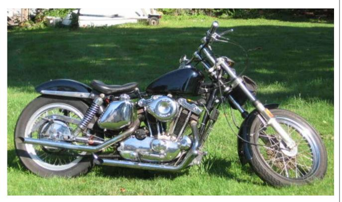
I have found that most bikes in this price range and era work best with some regular maintenance and are always great to ride. Recent new work includes .030 over S&S high compression pistons, new valves, valve guides, All Balls starter, Cycle Electric generator regulator, throttle and clutch cables.
