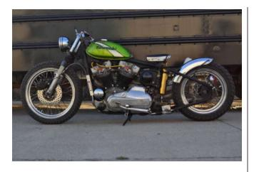
The bike uses no key, only a hidden very high quality, rubber sealed, made in the U.S.A. on-off switch. The carburetor on this bike is a retro-fitted, Italian made Dellorto.
