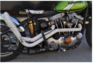
The hardtail is a K-model style tig welded with the continuous loop around the axle plates which is way better, and cooler looking in. It is quite a bit more expensive than your standard hardtail as well. The exhaust Ryan custom made out of aluminized steel j-bend header tubing.
