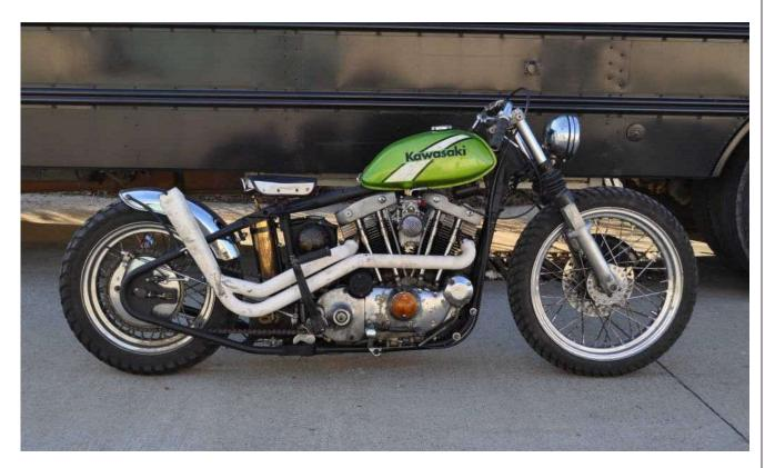
The bike looks old, but make no mistake, it is a fresh build. Its rough tough, and dirty as J Ryan intended it. It is inspired by the raw awesomeness of the flat-track and board-track bikes. The motor is mostly rebuilt with a complete top end bored .040" over with forged pistons. J Ryan completely rebuilt the cam chest with all new bushings, and shims, and installed high performance P-cams. The bike is pretty darn quick. Ryan went
