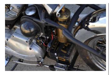
The mechanism is fully adjustable, in either direction. For normal braking you always want to lead with the rear brake. That's how Ryan has it set now. When braking normally its mostly rear with a little front, but if you push harder it will stop on a dime, utilizing the full capabilities of the front brake and rear brake.
