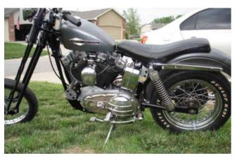
Front end is an original old Paugho front end and front wheel is an original 18-inch spool wheel with no front brake. Bike has original rear drum brake set up. All powder-coating professionally done by Lorac in Wichita, Kansas.
