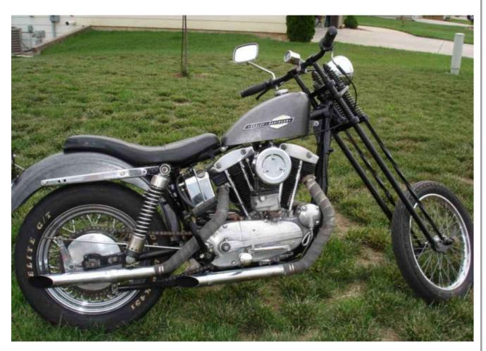
This is my 1966 XLCH Sportster. Lower end including crank pin, rebuilt rods, flywheels balanced and trued, new cams and cam bushings. Cases lapped and all new bearings. Transmission completely gone through and all case bushings lapped. Engine cases are mint and have no welds. Fins on both cylinders and
