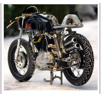
After the tank was completed, Carl fabricated the rear tank mount out of stainless. It was a difficult job, because he had to make sure that all nine mounts lined up in the right place. The end result was well worth the effort that he put into it.
