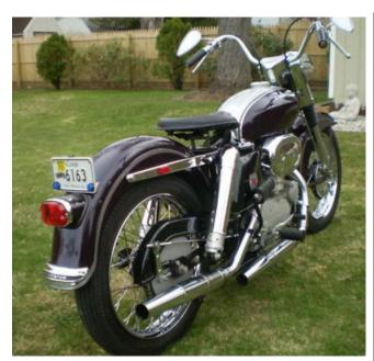
Rear chain guard is NOS and powder-coated. New chain front and rear. Seat is a solo with all the original hardware and springs. Rear shocks have been rebuilt using NOS shocks inside. Valve covers, clutch cover, cam cover have been bead blasted and cleared.
