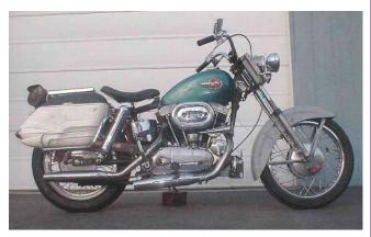
Here is a more recent shot of the bike after I fitted a valanced front fender and a 1959 tank. I also installed a beat-up set of Buco saddlebags.
