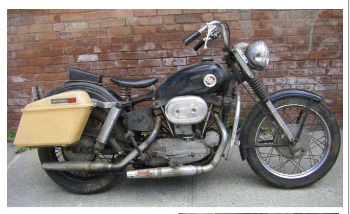
The trained eye can see this is a XLH engine in a XLCH frame. It's been together this way a very long time.
