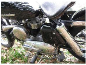
The cover in front of the shock holds the ignition coil and a tool-box. Brake is on the left, shifter on the right. This went until the 1974 Sportster, when the government mandated left-side shifters.
