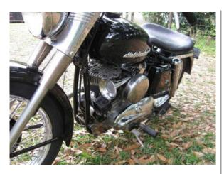
The trumpet horn is on the left side in K-models. So is the carburetor. The round chrome thing on the right side is the power pack for the horn, not an air filter. It does give the bike a nice symmetry.
