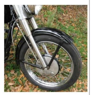
The early front end has "cow bell" covers over the fork tubs, not rubber "gators". Its a sleek clean look, no doubt inspired by the jet age. The brake was on the left side of the hub. The full-width brake came on 1964 Sportsters.
