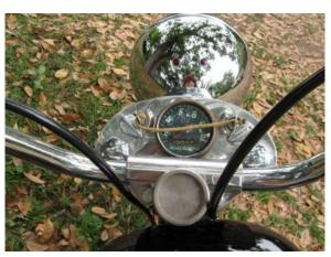
The dash has two keys, one for lights, one for ignition. The little swinging doors over the key cylinder are hard to find.
