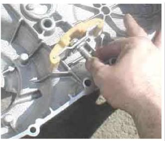
Back in goes the tensioner. Note the hollow part is out like when we took it apart. If yours is in the other way put it back together the other way. It's nice working on clean dry stuff. No oil to trap dirt and get your hands messy.
