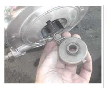
Slip on the magnificent ball ramp assembly. Notice the ridge where the hook mates so it only goes on one way. This has always been important according to the manual but I fail to see why the hook can't go on either way in a design sense. Only Harley knows for sure.
