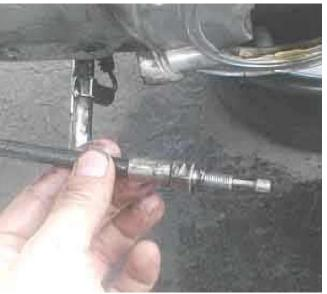
Another fine place for a leak. Make sure the little O-ring (what? No quad ring?) is in good shape and clean all this meticulously. Wham's funeral is only a couple hours away. Hope I make it on time.
