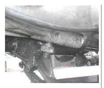
The chain tensioner won't thread out any further. It is not like the 1977 to 198? adjuster. Look further down and you can see the bolt is captive to the tensioner block. Just run the bolt out until you feel the resistance of it bottoming out.
