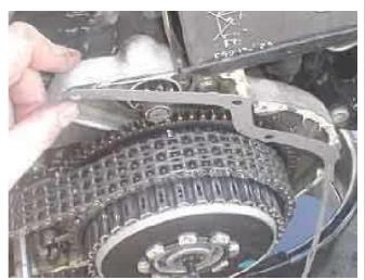
The gasket won't stay on the dowel pins. Brush on some assembly grease like I did and the gasket will stay in place even though it is pointed a little down.
