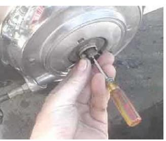
Where you can use a small screwdriver to spin the center bolt while the threaded hex nut assembly screws into the hex pocket on the ball ramp assembly. This is where you do the clutch adjustment. The factory says to tighten the center screw (by turning it counter-clockwise like you are unscrewing it) until you feel resistance.
