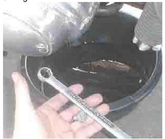
A 3/4 inch wrench takes care of the drain plug at the bottom of the motor. You might want to stand the bike upright after it has mostly drained out to get the oil that is sloshed into the primary cover. Harley never bothered to make the drain plug at the lowest point when the bike is on the side stand.
