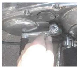
First remove the gear shift lever pinch bolt with an English size allen wrench. When I was an engineer with General Motors they had a firm target date of 1976 to convert over to completely metric. They should have asked the machine shops what they thought. Like GM cars today, Harleys are a mixture of English and Metric fasteners. Most of the big stuff is still English.
