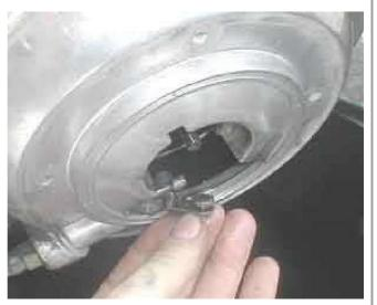
Here is the little hook thingy that wants to drop into the oil pan so bad. If you were not intending to pull the primary it would fall off inside the primary and make you pull the cover just to spite you. Toss it in the parts bucket.
