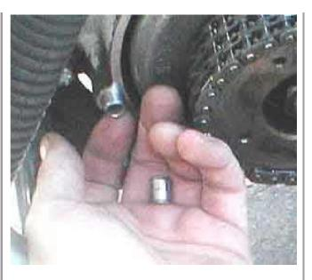
Back in go the hollow dowel pins, front and back.
