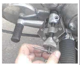
This bike was wrecked once and the gear shift shaft got bashed up a little. The lever won't slide off anymore. I use this totally cool little puller made for battery terminals. Please do not try to pry the lever off with a tire iron.
