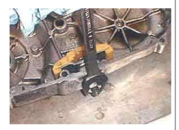
Go get the tool to remove the tensioner. A 7/8 wrench if I remember right.
