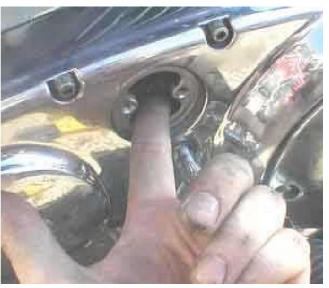
Feel the slack in the chain while tightening the adjuster bolt on the bottom of the primary cover. You should hit the starter momentarily to check at various places. My sprockets weren't out out round and the slack was the same. I wasn't brave enough to leave my finger in the hole while I cranked the bike. Don't blame me if your friends call you "Stumpy" when you loose a finger.
