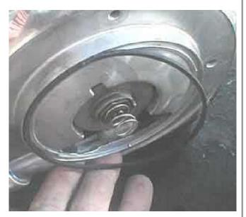
The spring thingy keeps falling on the ground and the quad ring won't stay put either. Sometimes the quad ring stretches and pops off one section, other times it compresses and pops off another.
