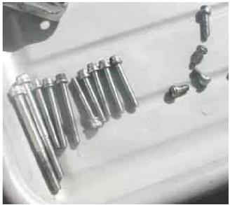
Note there are big bolts for the footpeg, long and short bolts for the cover, really short bolts for the derby cover and an oddball medium bolt for the shifter clamp. Don't be a wino and force the long bolts into the short holes.
