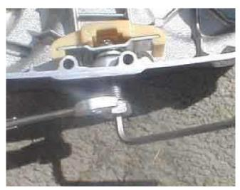
Of course the nylon makes the nut act like those evil prevailing torque nuts I hate so much. It won't free run in the bolt because the nylon needs to thread on the bolt for a (supposedly) leak free seal. Two tools. What joy.
