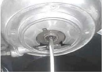
Screw the center bolt in clockwise to back out the incredibly beautiful release mechanism. Powdered metal I think. Must be great to have all that T-shirt money to over-design parts with. Forgive me, I still have a soft spot for the old stamped steel jobs used from 1970 to 1983. Now that was great design. Virtually frictionless and cheap as all get-out to produce. They probably early-retired that guy.
