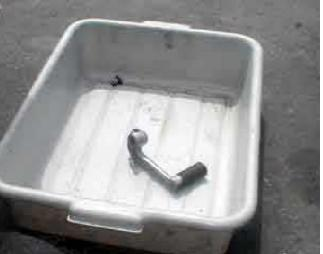
Use a tray to hold all the parts. The tray keeps all the parts in one place, it allows you to carry the parts to the wash bench and it can then be used for the clean parts. Carry it over to the polishing station and you will never loose a part. When all the individual parts are cleaned, polished, inspected for wear or damage and then repaired or replaced you have a tray full of parts ready to assemble.
