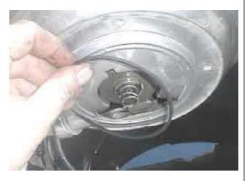
This is called a quad ring by the factory. It's kind of like an O-ring only it's square in cross section. I assume this will prevent us from using standard O-rings instead of official factory authorized original genuine big-dollar quad rings. Accept it and throw it in the tray with the rest of the parts.
