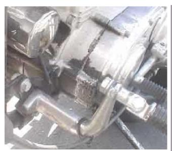
At about 12,000 miles a leak developed at the primary cover gasket. I had degreased and hosed the bike down the week before and driven it just a couple of miles before pulling over to look for the leak source. This is what it looked like after a weeks driving.
