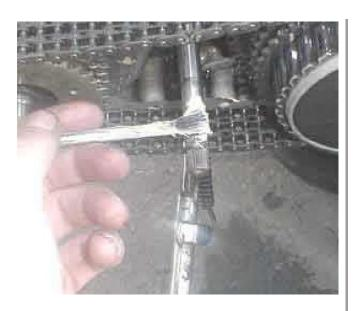
Put a little assembly lube on the gearshift shaft.
