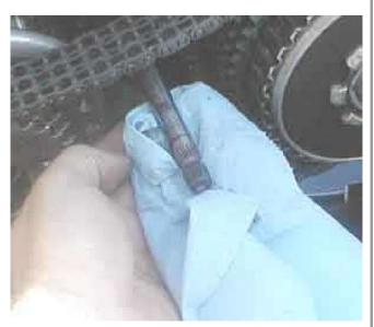
Clean the gearshift shaft. A lot of dirt can collect in the splines and it might be pushed into the primary when you slide the cover on. Cleanliness is the sign of a competent mechanic. I try to be so clean I don't' even swear when I put em together (although it's hard not to swear sometimes).
