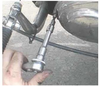
See, I can show off too. I do have a set of 3/8 drive Allen wrenches. It's a little handier but not a tremendous speed advantage over a plain wrench. I definitely use the wrench to assemble because it's shorter and bends a little to help judge the torque. It's no fun to strip these out.
