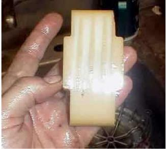
Notice how the chain runs diagonally to the tensioner. Be absolutely sure you put it in the same way it came out. As you can see from the picture above, the open side with the little hollow in the middle is facing out. The other side of the tensioner does not have this hollow.
