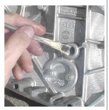
Put a little assembly lube in the primary cover where the shift shaft goes too. The factory says to replaces the shaft seal. If I had a seal handy I would have put it it. The splines are a little bunged up and could easily cut the seal up during removal.
