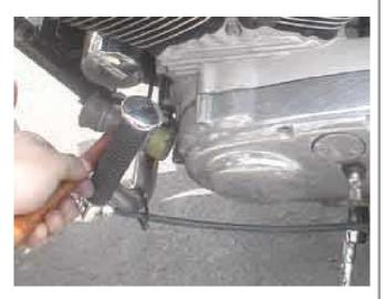
Unlike the 1970 to 1983 Iron Sportsters, the clutch mechanism has to come out of the evo Sportster to get the primary off. Note I just gave a couple taps with a soft mallet. I did not wedge a screwdriver in between the cover and the case which will cause an oil leak.
