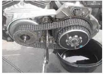
Behold the Sportster primary drive. Between the electric start setup and the demon-inspired alternator-behind-the-engine-sprocket, I'd say the chain runs a good 2 or 3 inches outboard of my '62. Notice how the starter bolts in above the clutch-- yup, you have to remove the primary cover to change the starter. Good thing Harley doesn't make cars. You'd have to unbolt the steering wheel when you change tires.
