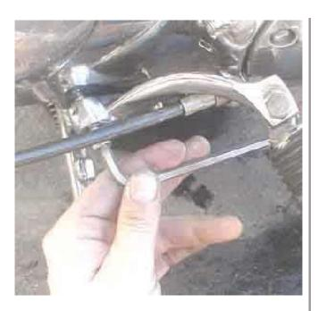
This is where panic turned to rage, The gasket did not line up for the footpegs even though all the cover bolts were in OK. I just leaned on the wrench to get the bolt to cut through the paper gasket. Horrible, this wipes off all the anti-seize. I'm sure I will be punished for this one day.
