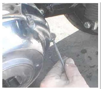
Get all the screws started and, unlike me, who will be suffering a few pictures later, start the big footpeg screws right now also. I didn't and the gasket partially blocked the holes. I was so late and I was so rushed I did not loosen the cover-- I just leaned on the wrench and forced the screws to cut into the paper gasket--shame.
