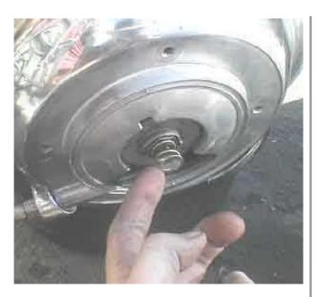
Pop on the goofy spring with lock disk assembly. If it keeps falling out just slather on a pound of grease and stick the dang thing there.
