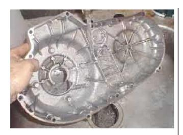
Wash the primary off with a lot of clean water. Blow it off with clean dry oil free air. Towels are bad because they leave lint but at least lint will be ground up in the bearings unlike silicone which will destroy any roller bearing. (Can you tell I like silicone?)
