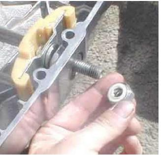
The tensioner lock nut has to go on now because it in interferes with the kickstand. Make sure the nylon surface is clean and free of all grit. Same goes for the area on the case where it mates.
