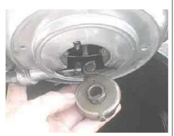
Out plops the breathtakingly gorgeous clutch release mechanism ball ramp sub-assembly. Stunning.
