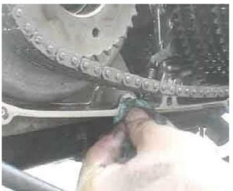
Clean the gasket surface perfectly. Do not scrape or nick or pry on it ever. If it is an old old bike that has been abused you can knock down any high spots with a fine file and build up any gouges with a polyamide epoxy like JB Weld. Under no circumstances should you use silicone or Permatex on the gasket. You should not have to glue your bike together. The silicone will get into the tranny and blow it
