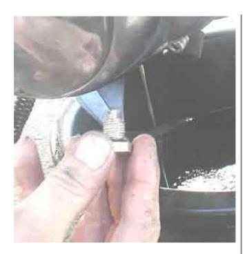
In the background we see 7 dollars worth of virgin oil draining into the pan with the old oil. Since there is no fill level plug on the late model primary cover I have to let the whole quart drain through. I have cleaned off the magnetic plug and blown off all the metal particles with air.
