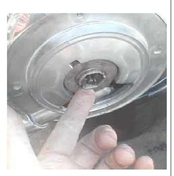
Swing the ball ramp assembly into the pocket....
