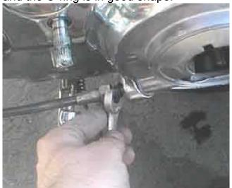
Be oh-so-careful using the wrench to start the cable. Get down on your belly and make absolutely sure the cable is going in straight before you begin turning. I got lucky this time and did not cross-thread and strip it out despite my being in a panic trying to get to my bro's funeral on time.
