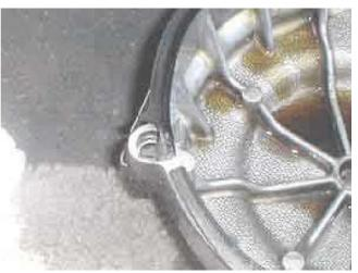
Here is the leak. It looks like the cover was over tightened. The Loctite on the bolts indicated that the cover had never been removed so this may be on the factory. On the other hand I bought the bike wrecked with 4700 miles on it and we know how those crank freaks like to tighten 1/4-20 Allen's with a half inch drive breaker bar with a cheater on it to boot.
