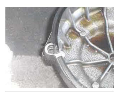
My 1996 Sportster keeps wearing through the primary cover gasket. Vibration and the footpegs being mounted to it must be the cause.
