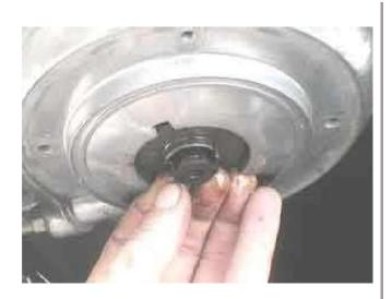
We're really jamming now as Frank Zappa would say. Remember that the problem is a leaky primary cover gasket? So here we are disassembling the clutch mechanism. Turn the center bolt enough and this little fancy hex-threaded gizmo pops out of the assembly. Thread it all the way off and toss it in the parts tray.
