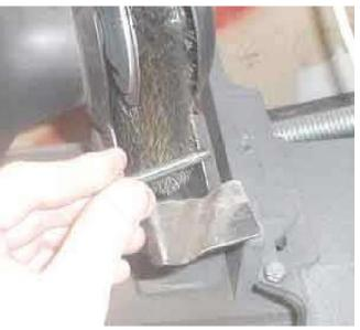
Get the crud off the threads. I just touched the wire wheel as lightly. As I use anti-seize on the threads as opposed to glue I don't think corrosion will be a problem. Please wear eye protection and hearing protection. The wires break off and can punch a hole in your eye.
