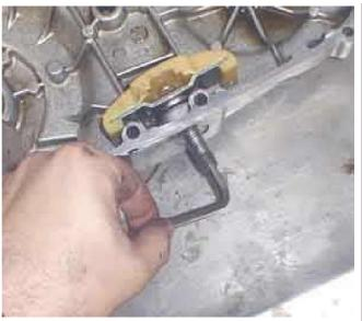
When you back off the big jam nut it goes over the grungy threads that were exposed to the elements and puts enough force on the center bolt to tighten it too tight to come off by hand. Go get the Allen wrench and break it free.
