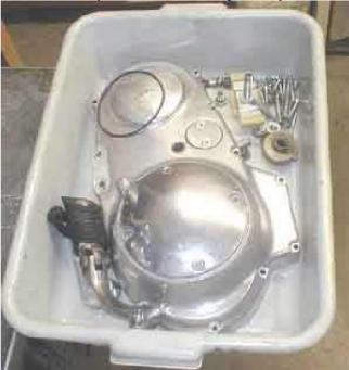
Here is our tray all washed out and cleaned and with all the parts stripped of oil, washed clean, blown dry and inspected for damage and wear.
