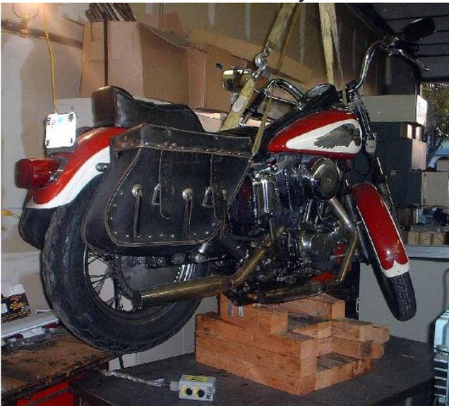
I get the bike up on the old desks I use to work on? A hoist on the roof beam. The desks legs are dropped into big steel tubes I welded casters to. I wheel the desk under the hoist, lift the bike and .....
