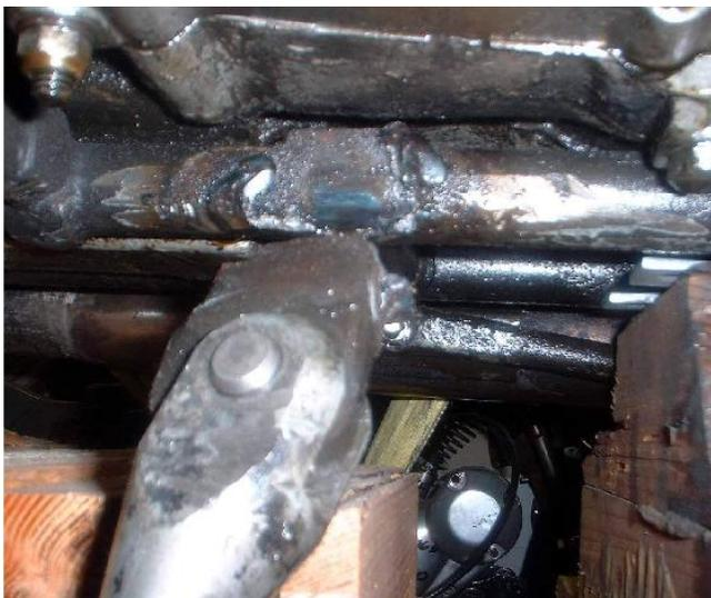
Here's a shot down under the primary cover where the side stand mounted. You can see the lousy weld.
