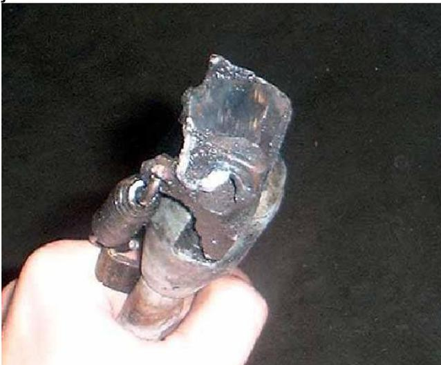
Here's a view of the first level clean up. Still a lot of work to do. There is a little undercut by the spring that I tried to bridge before, but now I decide to grind the undercut way deep so I can get a stick in there to weld the actual pad.
