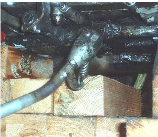
I bent the side side stand with a torch to make up for welding the bracket on at the wrong angle. My dad used to joke about golfers who had a bad slice "fixing" their slice by just standing at an angle to the fairway. They still sliced, only the ball went down the fairway kinda sorta. Same stupidity here. I should have ground of the bracket and started over. Actually the real cool way to fix this is to pull the motor.....
