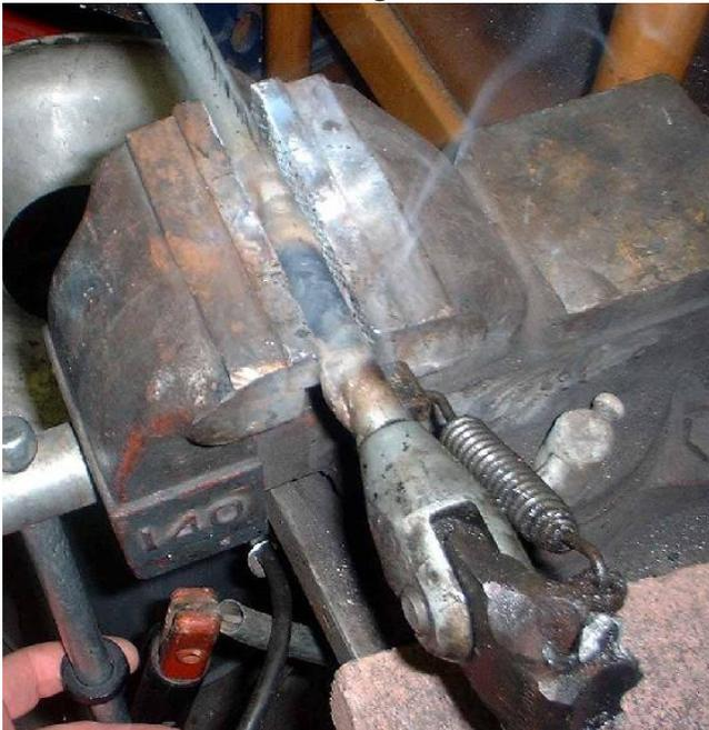
While it's still red hot I clamp it hard in the vise twice at 90 degree rotations to straighten it that last little bit.
