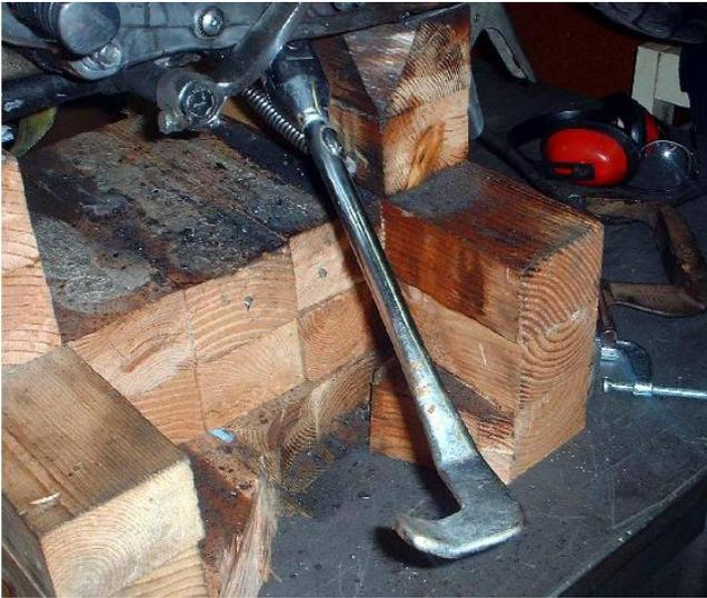
The screw still didn't want to thread in even after I chased all the treads. I went into the parts stash and found this nifty jiffy stand I scored at a swap meet. It's a bit longer so I figure if I did weld the bracket in perfectly this will compensate for the 21-inch wheel in the front. It's also got the little tab on the end that makes it a lot easier to find the stand with your heel.
