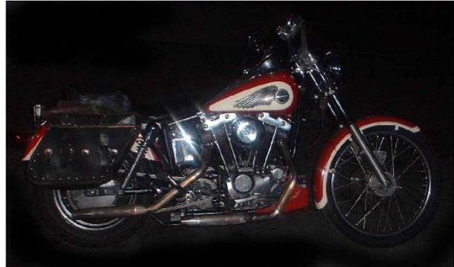
Here's the show side of the bike. I threw the sprocket cover in the trash and fabbed up a steel bracket for the kick starter. I mount the battery in the front in that swoopy bracket you can just make out. I need to redesign it though-- this fender just touches it at full jounce. That's a project for another day.
