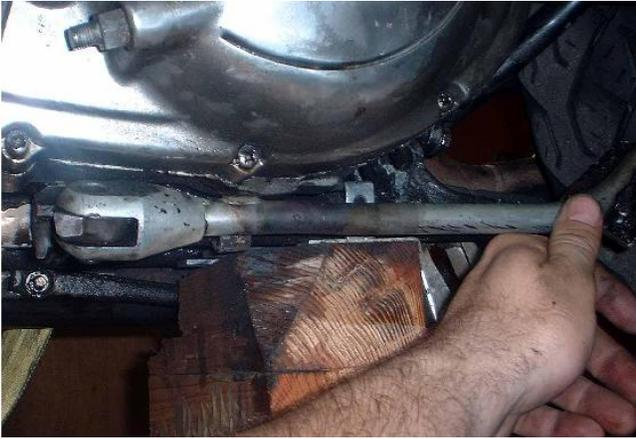
Here I swing the stand back and see how it looks in the up position. It looks much better than it used to with that bent stand. It is a little low but it almost stops in the exact same dent the original stand did 25 years ago. After this looked OK I just ran the stick around the bevels. It's like paint--days of preparation minutes of painting. The actual welding took about 20 seconds. It was still a little splattery so I won't shame myself with a picture you decent welders will laugh at.
