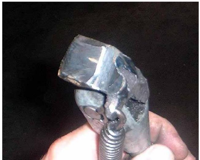
I really got medieval on this thing. You can see where I ground the undercut way way deep by the spring so I can get in with the stick welder. Also notice the bevels on all the three sides that I will be able to reach with the engine still in the frame. My buddy. Phil was the guy whose dad used to say: "Everybody wants to **be** somebody. Nobody wants to **become** somebody." I don't know if I'll ever be a welder.
