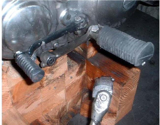
My welding lasted six months before the bracket broke off again. This looks a little strange for an iron Sporty. My 1977 has a 1995 primary cover with the starter pocket cut off and welded up. I run a 57 to 66 dry clutch setup with a custom lever/ I welded a foot peg mount on the 77 frame so I can run the 76 and earlier foot pegs instead of the engine mounted foot pegs. I run a 73 and earlier right-side shifter on the cut down shifter shaft.
