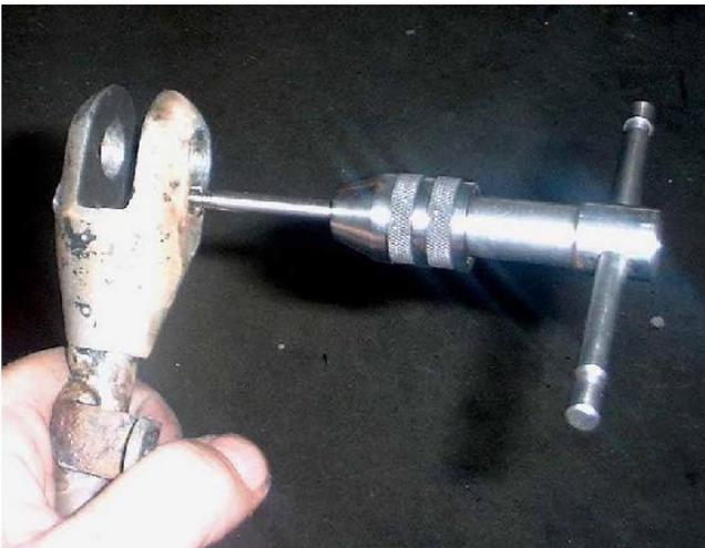
Always misery and suffering with Harleys. I guess it builds character. The little stop screw that holds the pin in won't thread in easily. I clean up the the threads (12-24) and run the screw into a die
