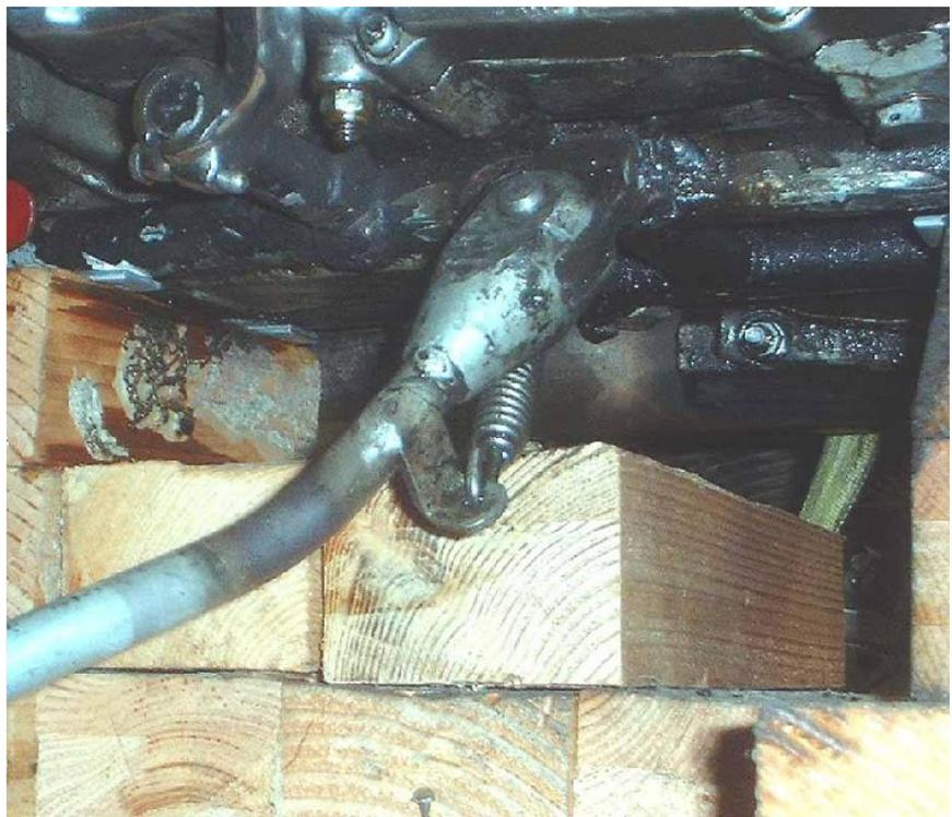
The Sportster sidestand bracket takes a lot of abuse on a kickstart-only bike. This one has broken off after a bad welding job.
