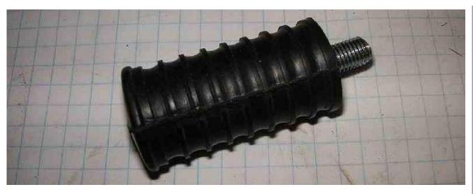
Here is the repop shifter rubber. Flash from the molds, crappy soft rubber, and no "Harley-Davidson" molded into the rubber.
