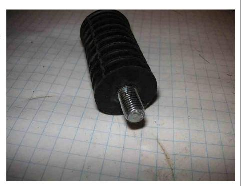
Here is the stud, the factory manual shows that the threads don't go all the way to the rubber. This one threads into the threaded parts of the lever. The factory lever has the non-threaded hole and you use a nut on the stud.
