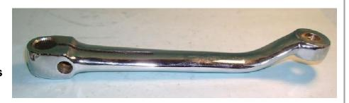
The first two years of the K-model take a shift lever that has splines where the shaft goes. This is the same as the lever used in the WL 45-inch flathead.
