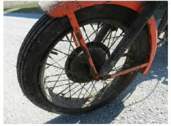
Here you can see the correct side-mounted brake drum. I think the fork sliders are supposed to be cadmium plated. Maybe they are under that black paint. This must have been in a barn. A bike left outside gets way rustier.
