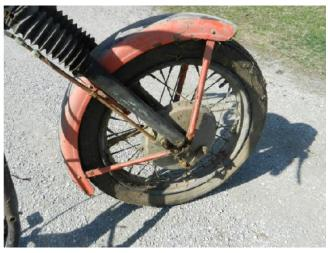
The fender is Sportster. See how the struts have a 2-inch flat spot where they attach to the fender? That is to accommodate the valenced fender that has side panels. K-model fenders have the rounded strut go all the way to the fender. All kinds of nice parts like the brake tube, adjuster, brake tube fender clip, lever and shackle. The front end has the bellows. A 1952 is supposed to have "cowbells," steel covers that mount on the underside of the triple tree.
