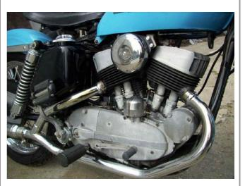
The 1952 K-model engine is only 45 cubic inches (750cc). In 1954 Harley introduced the KH model, with a stroked flywheel. It boosted displacement to 61 cubic inches (883cc).
