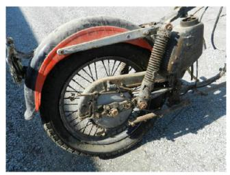
The brake switch is not supposed to be on the chain guard, it goes on the back of the engine primary cover. This is very coherent with this being a KR race bike, The flat-tracers did not use the stock primary cover. Oops, the strut bolts are Phillips head, that's not right. Brake rod is there, nut on the rod, lever is correct. Axle and shock hardware are there and looks correct.
