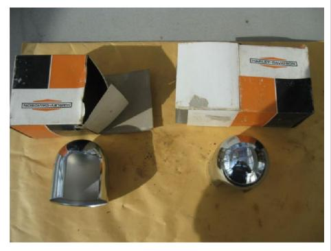
It is always nice to run these covers so that when the kickstarter slips your leg does not slam against the sharp shock mount and nut.
