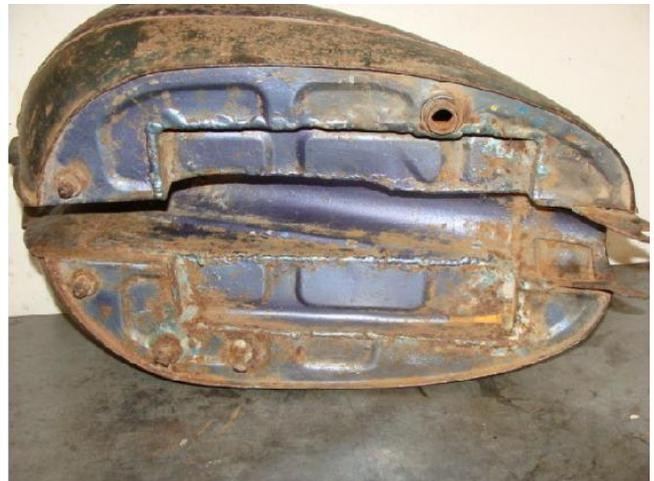
But look at this hack job. Someone has cut the bottom of the tank and recessed it so it fits on a Sportster. Now maybe this is just me, but I would rather just weld back the tabs on the red tank I bought. Heck, you can use double-face foam tape to hold the badges and trim. V-Twin makes a repop of this great tank now, and that is my plan-C, if I can't get one of my two tanks working. With this tank you will be in constant worry that the crappy welds will spring a leak.
