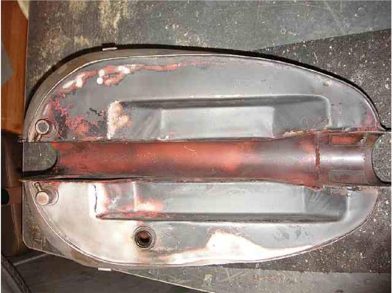
Oh, in case you want to see how a real Sportster tank is made, here is a picture of the bottom of a 1957 Sportster tank. The outer shell is the same, other than
