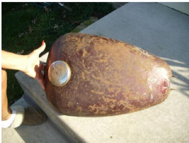
The dents in the tank are the reason it was put in the junk bin. That's a better situation than if the tank was rusted out with no dents. Everybody tells me to use Kreem or the POR stuff to seal tanks. Sorry, that is just epoxy paint, and it never works. At least not in the long term. Ask my buddy Angel, whose Shovelhead would stall when the sealer peeled off in sheets and clogged his petcock strainer.
