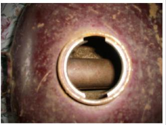
The tank looks pretty good inside. Thing is, they don't rust out here, its at the rear where the water collects. Now that the farm lobby forces us to have a bunch of corn ethanol in the gas, the tanks will rust out even faster. Alcohol is hygroscopic, it absorbs water from humidity in the air and holds it up against the metal inside your tank. I hear there are "no ethanol" gas stations popping up all over the country. The alcohol also swells and ruins the rubber and the seals in your carburetor.
