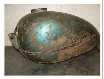
Here is the left side of the K-model tank that went for 1000 dollars. Pretty nice and it has the strip mounts. A lot of guy ground these off in the chopper days. I later bought a red K-model tank like this.
