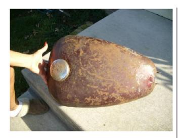
The dents in the tank are the reason it was put in the junk bin. That's a better situation than if the tank was rusted out with no dents. Everybody tells me to use Kreem or the POR stuff to seal tanks. Sorry, that is just epoxy paint, and it never works. At least not in the long term. Ask my buddy Angel, whose Shovelhead would stall when the sealer peeled off in sheets and clogged his petcock strainer.
