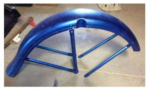
You can see the nice flare on the rear of the fender. My K-model rolling chassis came with a front fender, but it is the 1959 Sportster strut fender.
