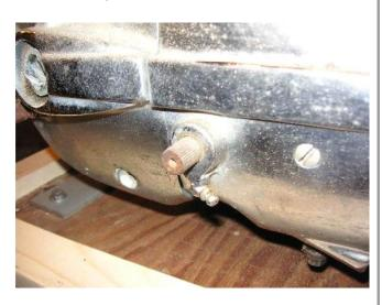
Here is the shifter shaft. It does not look bent. Note that it is splined. I had a smooth bore lever that fit over it, but then got a splined one, I think aftermarket. Note the ultra-cool angled Zerk grease fitting at the bottom of where the shaft comes out..
