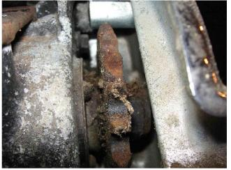
The sprocket looks to be in pretty go shape. I have taken to putting a new sprocket on with every new chain. The sprocket on the brake drum can last for a while, but the small tranny sprocket gets worn pretty bad, pretty quick. A worn sprocket will ruin your brand new chain in a few miles. Thing, is this 1952 sprocket may be different than the aftermarket and factory sprockets for Sportsters.
