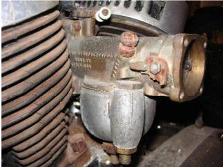
The carburetor was included which made me feel \$2500 was a fair price. It is probably the real carb that came with the bike in 1952. That, the generator, and the fact that the motor was not in pieces inside a peach basket. The Linkert looks corroded, but bead-blasting will amaze you. [I have since decided to not bead-blast the carb. I think I will ultrasound clean it.] That cylinder base nut looks just like the ones on my 1979 Sportster. Its the longest-running motorcycle model in history.
