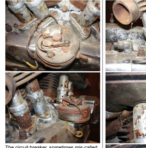
The circuit breaker, sometimes mis-called a distributor, is rusted badly. Harley interchangeability means I can slap in an auto-advance circuit breaker. This one you advance and retard by hand, with a twist grip on the left side of the handlebars.
