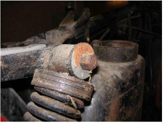
The eBay listing showed the double groove on the shock. That is just like the 1952-53 shock in the parts book. I am pretty sure the studs, nuts, and washers are all available repop, in "cad". I don't know if that means "zinc" or cadmium. I am pretty sure I can get the rubber bushing new as well.
