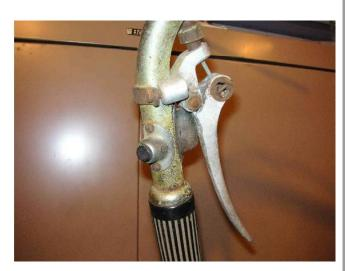
Here is another money shot. The lever, the switch, the pivots and even the screws, all this is original an all is treasure. I think I saw a local Tampa shop that does cadmium plating. That would be great for a lot of parts, but many plating shops won't do automotive parts, since they are used and might ruin the plating bath.
