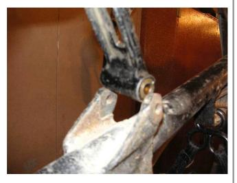
Sorry for the crappy picture. Someone reefed down on the seat mount and bent the frame so a factory seat T will not fit. I figure a torch and a nuts on the inside of a threaded rod might flex it back out.
