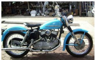
Here is a restored K-model from over in the Smorg section of the website. This chassis was a huge advancement for Harley. The K-model was the first bike to get a rear suspension, and in 1952, long before the 1958 DuoGlide. The chassis does retain the sprung seat, like a big bike or 45 flathead.
