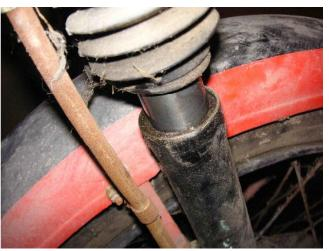
Here is a nice surprise. The fork tube is not rusted where it counts. I am pretty sure these tubes have seals in them, which means the are meant for the tin "cowbell" covers, not the rubber "gaitors". So maybe this front-end is a 1953 like the frame. Nice.
