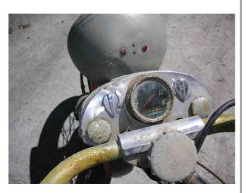
The eBay ad had a big shadow that covered the dents in the top tin. But I could see it was real Harley top tin. The little pear-shaped swivel lids over the ignition and light key-switches is Harley, the repops are flat. The real tin also has the indentations for the flippers. The dent will be easy to pound out. But the eBay picture with the shadow also hid the speedo face. It is in much better shape than I expected. That us a big deal, speedometers can cost 500 bucks.
