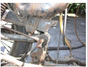
Everything looks OK here. The brake is even adjusted right, so the pivot lines up with the swingarm pivot. That way when the bike rear suspensions jounces or rebounds, there is no change in the position of the brake rod relative to the drum.
