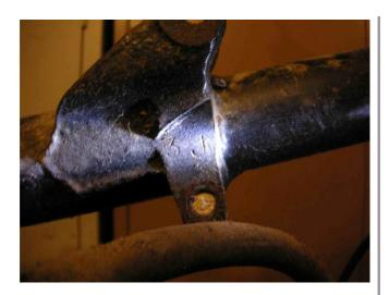
Now that the bike is up in the air, first thing is to see what year the frame is. The top motor mount made it clear it was K-model, but that could be 1952-56. This is the right side of the seat mount, where the gas tank mounts. The 3 means 1953, the J is the 10th letter in the alphabet so that means this was made in the 10th month of 1953, October.
