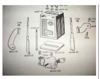
Here is the battery page of the 1956 K-model parts manual. It shows two 66404-52 straps that you need for the 66224-52 part, but also the bolt with cross-pin you need for the -B part. This picture is of Harley Davidson copyrighted material.
