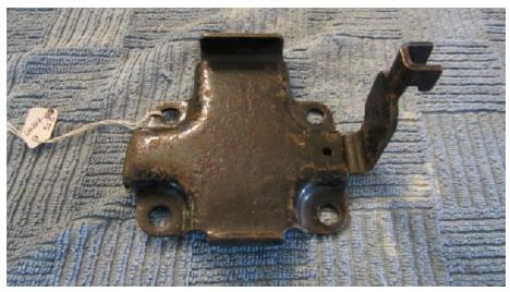
Here is the 66224-52B battery carrier. It has a welded bracket that takes a bolt with a cross-pin. The other side takes the same strap as the 1952 part.
