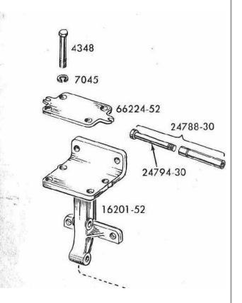
This is on page 6 of the 1952 K-model parts manual. It has the right battery carrier part number but I have never seen a part like this. It looks like it is supposed to have longer bolts with cross pins. This picture is of Harley Davidson copyrighted material.
