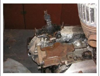
Here is this 1954 bracket alongside the 1952 bracket that is on top of the motor mount. Note I have the 1954 bracket reversed, the vertical tab is on the right side in the parts book, see next pic.
