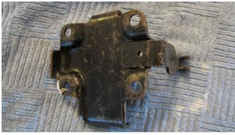
Here is a bottom view. This part piggybacks on top of the steel rear motor mount.
