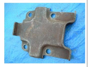
Here is the correct battery carrier for a 1952, part number 66224-52. It also picks up the back bolts on the motor mount. Holding tight tolerances over a sheet-metal bend is hard, I can see why Harley changed the part. I bought this a few weeks later. I will have a post for that as well. I will sell the wrong one and recover some of the cost. I looked at all my parts books and I can see why the seller said this was for 1952 K-models. First off, the 1952 book is schwacked.
