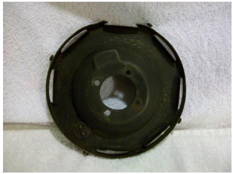
You can see the missing section at the top of the backing plate. The seller was honest, he made sure to point this out in the listing and the pictures. To show how the filter sits on the bike, you would have to rotate it clockwise a bit over 90 degrees. That rectangular bump by the carb hole is to clear the choke. The circular tab at 7 o'clock is the backing for the horn mount tab. It is riveted on.
