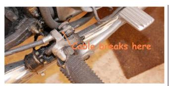
Your brakes are critical. I once had both brakes fail. It was that crappy rear cable used on 1974 to 1978 bikes, and a bad gasket on the front master cylinder. It feels really weird riding a bike with no brakes. You can coast down with the clutch pulled and scrape your feet to stop. I suspect killing the engine and letting compression slow you down works well too.
