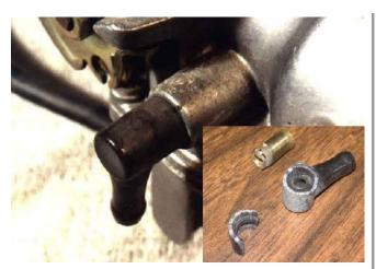
All Keihin carburetors crack and leak at the inlet elbow. My 1977 cracked and leaked, my 1996 cracked and leaked.
