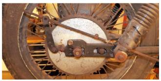
My common failing on old Sportsters has been to over-tighten adjustments. I would tighten the brake rod adjustment so the pedal would move only an inch or two. But the shoes dragged and the backing plate was so hot after a ride it would boil water.
