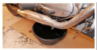
Ahhh sumping. When the bike sits for a long period, and you start it, oil blows out the breather tube. 1976 and earlier bikes will often have oil leak past the oil pump so all the oil in the tank ends up in the bottom of the engine. There is a springloaded steel ball that is supposed to stop this. There are also seals on the shaft and I suspect worn gears can make the problem worse.
