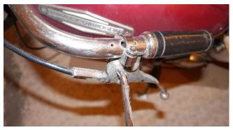
The dry clutches adjust the cable up at the bars. I use Barnett steel levers since they have a tiny bit more travel. They also just bend when you drop the bike, as opposed to breaking off.
