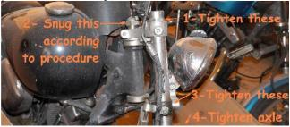
Read the service manual carefully, and buy the factory manual for your bike. In general, you tighten the fork tubes to the top triple clamp but leave the lower clamp loose. Then tighten the fork stem. You have to have the bike up in the air. The axle should be loose too. I tighten the stem until the fork still flops to the side under its own weight when it is half-way turned. It has to be this loose or you might dump. Once you get this, tighten the triple tree and the axle.
