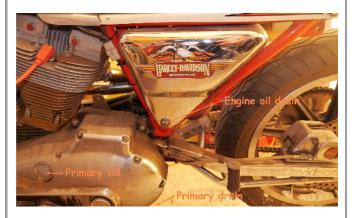
There are two separate oil systems in an Iron Sportster or K-model. The engine oil is in the tank. There is a drain on the tank bottom. Then there is separate oil in the primary and transmission. You drain this with the plug on the bottom of the primary cover (left side). There may be a plug in the bottom of the crankcase but that should stay put, it does not drain anything unless the motor is sumped.
