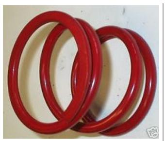
A buddy had his clutch drag on his 1974. A mechanical had just put in a new spring. This was a single "heavy duty" spring. You need the two factory springs to keep the clutch plate level as it gets pushed in from the center. You rotate those two springs until they apply an even force. This two-spring setup is a mistake compared to the 6 separate springs of the dry clutch. We are Devo. D E V O
