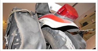
So realize that wires are a simple, stupid, but critical part of the bike. Check back there under the rear fender, and look around the fork neck as well, where wires get bent in day-to-day use. Wires can fray inside the headlamp bucket and I had a 60W halogen bulb melt the connector. Anytime you change things from dead stock, you risk these kinds of problems.
