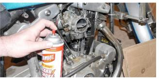
I blew up my 1977 because it had an intake air leak. The leak made the front cylinder run lean, and that burns a hole in the piston. To check this, spray carb or brake cleaner or pretty much anything where the intake O-rings are. It the engine speeds up or slows down that indicates a leak. Be careful to not let overspray into the air filter or you will get a false reading.
