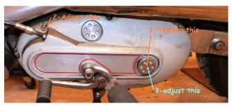
The clutch is another thing that likes it a bit loose. The dry clutch has to be set up loose or you will wear out the rods in the mainshaft. The procedure makes sense about the 40th time you do it, see the manual. You need to adjust for the length of the cable first, then you adjust the clutch itself.
