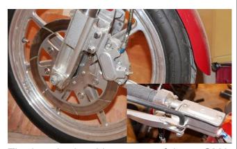
The best brakes I have every felt are GMA brakes on my XR-1000. The worst brakes I have had is with the Arlen Ness chopper master cylinder. It's reservoir is too small and DOT-3 makes the piston swell and seize up.
