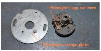
The 1970 and later cone motor has the ignition flyweights on their side. They beat themselves loose at the pivot. Then the weights clank against the underside of the breaker plate until the 1/4-28 bolt shears off, flush with the camshaft. Even the 1979 electronic ignition uses the weights, it was only the module electronic ignition that did away with them. Some bikes are worse than others for how quickly the weights get egged out. This is something you have to check often.
