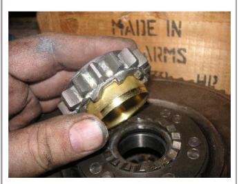
I used to hold in the clutch at lights. I figured it saves the gear dogs getting clanked. Well, on dry clutch bikes it wears out the thrust bearing in the clutch basket. See the big thread on the XLForum.
