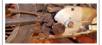
The rear brake has an adjustment for the pivot too. In theory the clevis where the rod attaches is supposed to be centered with the swing arm pivot. I will let you argue as to where that is with the brake engaged or not. One way reduces wear, the other means the pedal does not pump with the rear suspension jounce.
