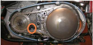
There is also a transfer valve in the primary (1, 2, 3, 4). If the bike is sumping and this valve is bad, then the excess oil overfills the primary and transmission.
