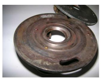
A close-up of the plate shows how badly the advance weights have worn it. The plate might still work, but you have to replace the advance weights, or maybe just replace the whole setup. I have not tried the aftermarket needle-bearing unit.
