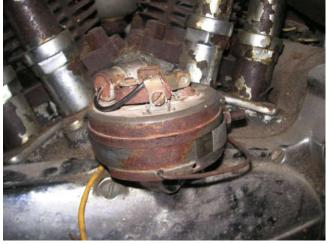
From 1952 to 1964 the engine had a cable-adjusted advance circuit breaker.
