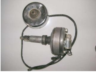
In 1965 the cable advance was replaced with a circuit breaker with automatic advance weights in the base. It seals with a O-ring to cam cover. This unit has the optional tachometer drive on the cover.
