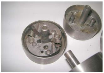
I designed a plate and cup so that the weights would not twist when flung outwards. It used the pivot pins from the old plate, and I drove the roll pin out of the weights. It was a total failure, the weights would bounce off the hard steel cup and the bike would run terrible the second it came off idle.
