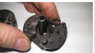
A bad weight set with the pivot egged-out so the weight lifts up.
