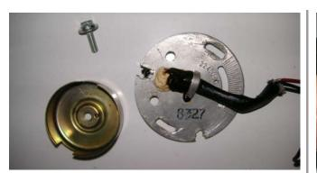
In 1980 the factory put a sensor only inside the cone, and a module on the frame under the seat area.
