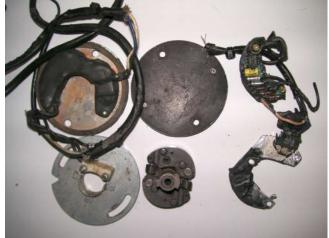
In 1979 only, Harley used an electronic ignition but kept the troublesome advance weights. Having electronics in the hot cone means less reliability, but even less reliable is the mechanical advance.
