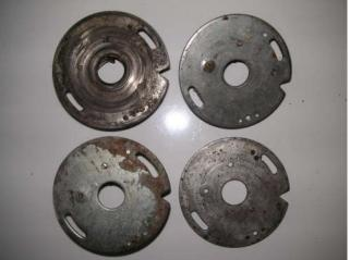
The top-left plate has had the advance weights hit. There are deep grooves worn in that plate, compared to the other three plates. The constant impact will eventually break the 1/4-28 bolt, shearing it off right at the camshaft. Use anti-sieze on the bolt so you can work out the broken piece with a scratch awl. No Loctite, ever.
