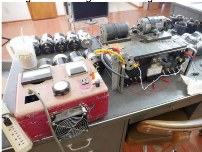
The test rig with power supply (left), motor-generator, and load box.
