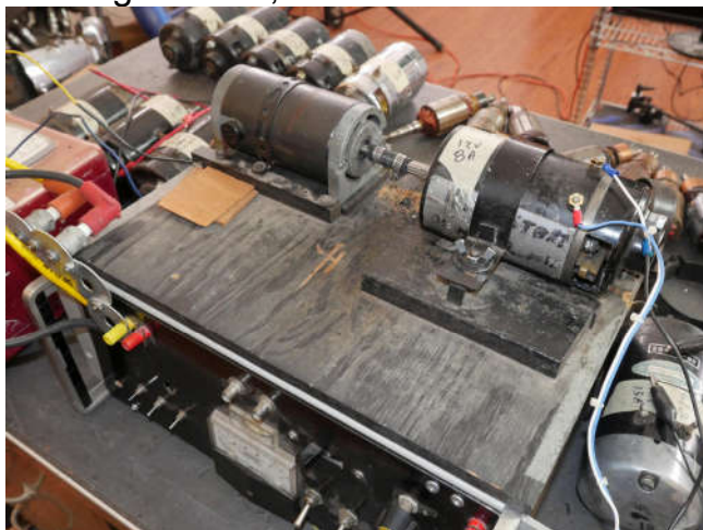
The motor driving the generator comes from a salvage yard. It is a 115V DC brush permanent magnet motor. A rubber hose hooks it to the generator under test. The plywood base sits on a load box.
