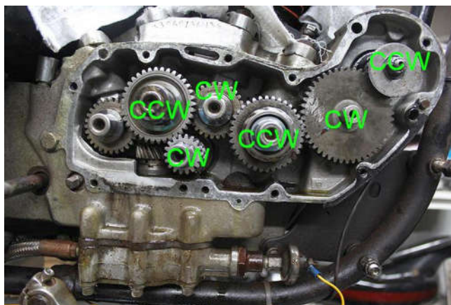
Sportster generators turn counter-clockwise when looking at the drive shaft.
