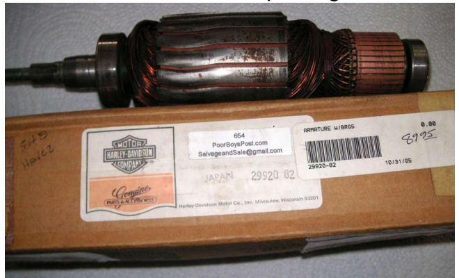
There are factory NOS replacement armatures available, way nicer than the aftermarket units you get when buying a Model 65A armature.
