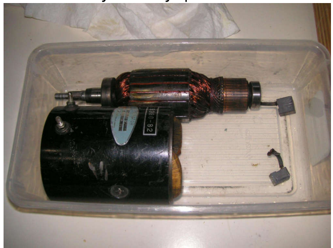
The cleaned parts that did not go into the solvent tank. I did bead-blast the armature, since it is junk anyway.
