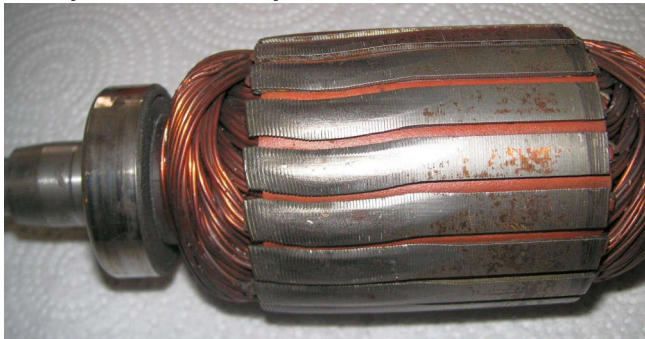
I blasted the armature since I have never ever seen the lamination get beat into a spiral. This generator had a bolt missing. I have to think the armature was hitting the pole shoes and got beaten into this state. The astonishing thing is the generator still worked. You can see the diameter of the armature is smaller on the left side. Unlike the -65A generator, this armature comes with the bearings pressed on already.
