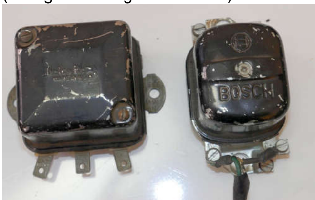
The factory used the Delco-Remy regulator on coil-ignition bikes, and the Bosch on the right in XLCH kick-starts.
