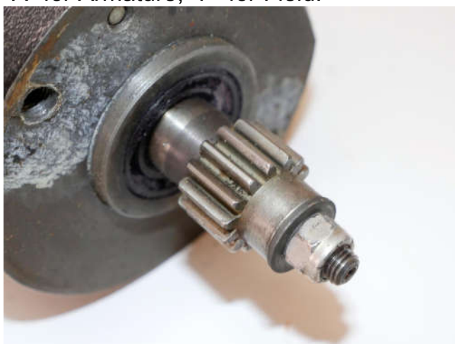
The drive gear is carryover from the -65A, but with a small flat-washer instead of the large oil slinger washer. Same nut is used.
