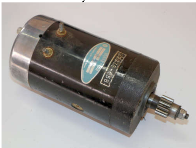
Like older generators, the terminals have "A" for Armature, "F" for Field.
