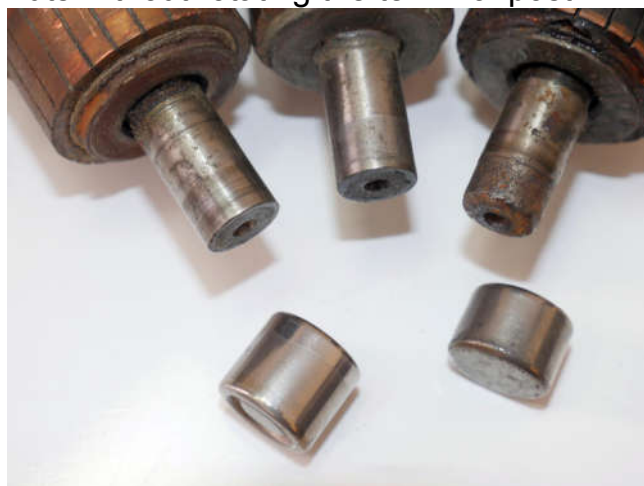
Rebuild kits come with needle bearings. The left shaft is OK, the middle and right side ones are junk, get a new armature.
