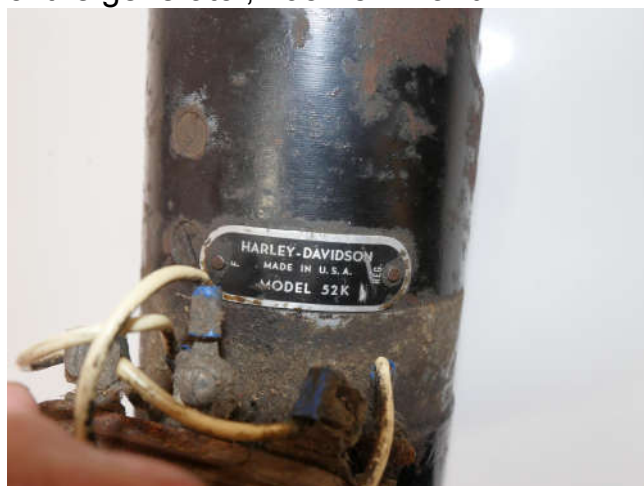
The riveted tag identifies this generator as a Model 52K.
