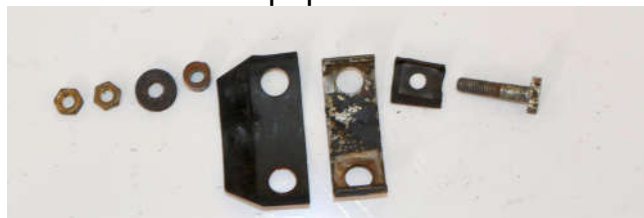
Here is the terminal plate laid out so show the square paper washer. You can fix this without disassembly by loosening both nuts, rotating the terminal with needle-nose pliers, and carefully re-tightening the nuts without rotating the terminal post.
