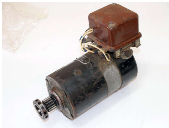
The 29982-52 mounts the regulator on top of the generator, 1952-57 K and XL.
