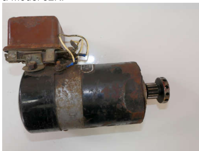
There is a divot in the frame to clear the engine case. The generator is for 6-volt motorcycle electrical system only.
