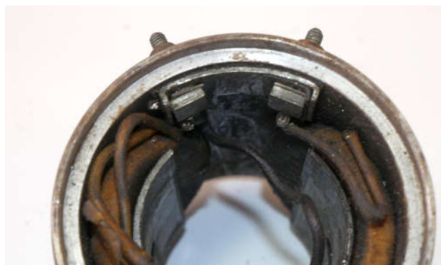
The -65A generator and most likely earlier 6-volt versions other than the -52K have a design problem. There are small square paper washers that insulate the square head of the terminals. If someone over-torques the terminal, the corner of the head can cut the paper and short out.
