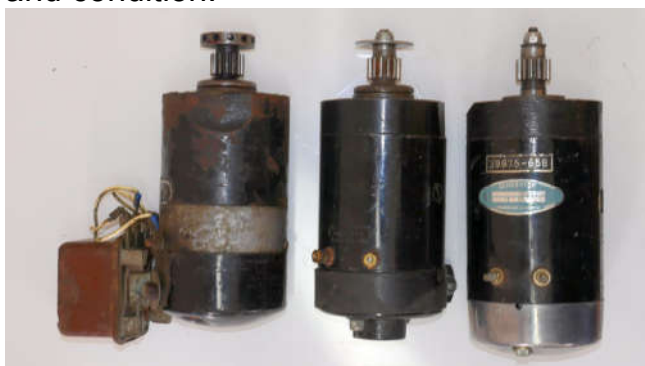
On the left is the 6-V Model 52K, part 29982-52. There was a Model 58 variant, 29975-58, similar to the middle picture but with oil cups on a plain armature bushing. The Model 61, 29975-58A has needle bearings and no oil cups. The middle is a Model 65A, 12-V, 29975-65A. There was a 29975-65 for 6 months. Right is a Model 65B, 29975-65B, also 29978-77A
