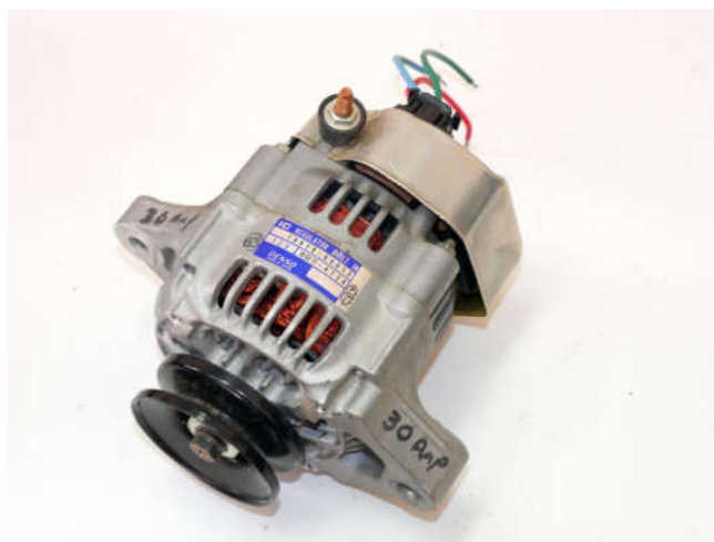
This car alternator fits in a Sportster, a machinist made an adapter drive for a few years.
