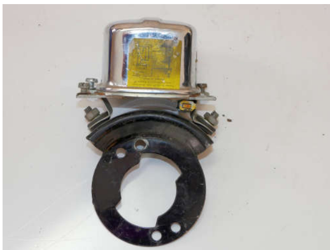
The Model 58 generator mounted the regulator with this bracket 74524-58 (wrong Bosch regulator shown).
