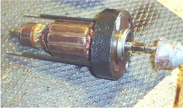
Gently tap armature out off the end bell with a small rubber mallet. I really mean rubber-- if you use a regular hammer you will mash the threads on the end and life will be difficult. If you must be a wino at least thread the nut back on the armature and pound on the nut.
