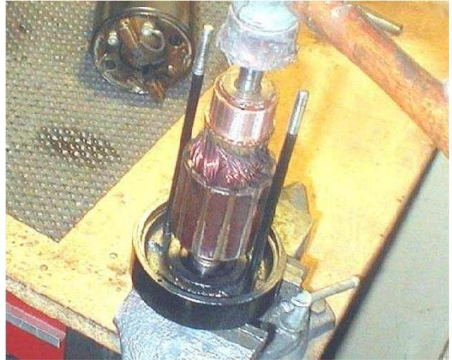
Tap the armature in with a small rubber mallet. The vise is opened up and gently tightened on the protruding rings of the end bell. You aren't supposed to use sandpaper to shine up the copper commutator because the grit gets stuck in the soft copper and then grinds up the brushes prematurely.
