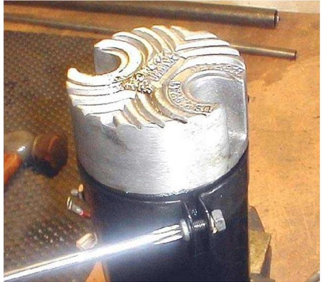
Now you can tighten the brush cover. This one is eye-balled so it points down when the generator is installed. This area was where the oil was coming out.
