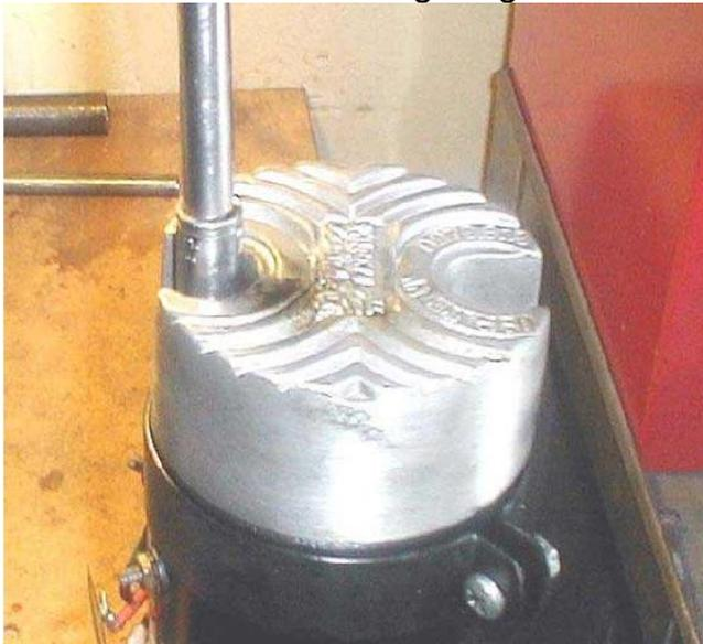
Because of the regulator I needed a deep well socket. Otherwise a 7/16 wrench will work. Always replace the lockwashers--even if you tightened it and then had to take it back off for some reason. Then you will not have to glue your bike together with Loctite. I replace the nylon prevailing-torque nuts the factory uses with regular nuts and lockwashers.
