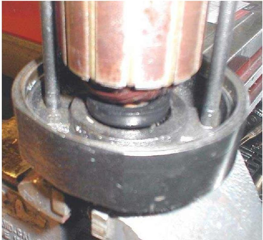
The Harley 12-volt generator has a seal in the housing that bolts to the engine case. This seal has popped out due to pressure inside the gearcase from a sumped engine.
