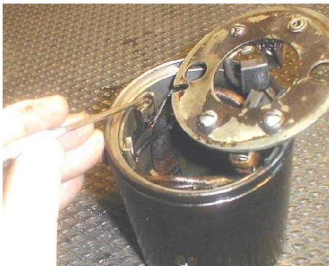
Look carefully at the little paper spacer under the square head of the field terminal. If the terminal was torqued too hard this thin paper gets cut and the field gets shorted to the armature and the generator has no output. There are some plastic spacers around. Anything including the plastic from a milk bottle is better than nothing. If you tighten the terminal up carefully you can insure the corner of the square head is not cutting through the spacer.
