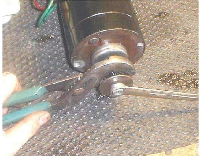
The gear will only start on the shaft as it is a light press fit. Some gears do just slide on. The Factory uses a nylon prevailing torque nut. I substitute regular 5/16-24 nut and a pair of the trick Disk-Lock lockwashers. A real touch here as you need to feel the subtle difference of the gear pulling on and, once it all the way on, the increase in torque as the nut tightens. These 5/16-24 threads strip easy.
