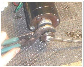
The gear will only start on the shaft as it is a light press fit. Some gears do just slide on. The Factory uses a nylon prevailing torque nut. I substitute regular 5/16-24 nut and a pair of the trick Disk-Lock lockwashers. A real touch here as you need to feel the subtle difference of the gear pulling on and, once it all the way on, the increase in torque as the nut tightens. These 5/16-24 threads strip easy.
