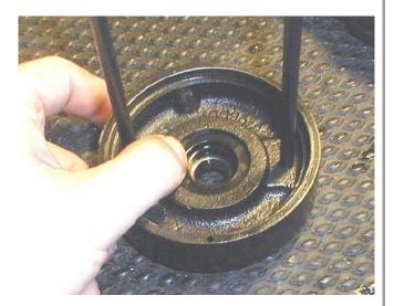
The seal was still in good condition. It just popped back in with finger pressure. You could use a tiny tiny tiny bit of Loctite or Permatex on the outside of the seal but be extremely careful. The tiniest bit of sealant can get into a roller bearing and start jamming a ball, making it skate instead of roll. Silicone and gasket sealant cause horrible damage in a roller bearing engine.
