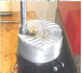
Because of the regulator I needed a deep well socket. Otherwise a 7/16 wrench will work. Always replace the lockwashers-even if you tightened it and then had to take it back off for some reason. Then you will not have to glue your bike together with Loctite. I replace the nylon prevailing-torque nuts the factory uses with regular nits and lockwashers.
