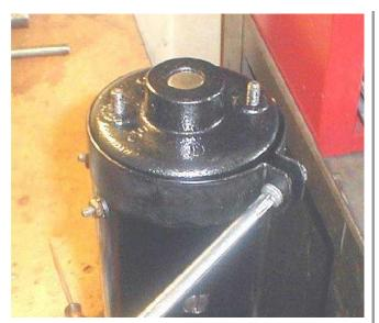
cool air into the generator. It worked great in the rain, everywhere for 5 years. Until I blew a front fork seal and the fork oil splashed on the commutator. It glazed it over and ruined the voltage regulator.
