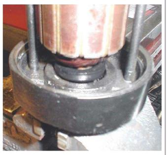
When the old '62 sat for a month the motor sumped. This means the oil in the oil tank leaked down into the motor. When I started it all the oil was forced into the gearcase. A bunch of oil blew out the gearcase breather tube but the pressure got high enough to push this oil seal out of the generator. Oil leaked out the generator every time I ran the bike since.
