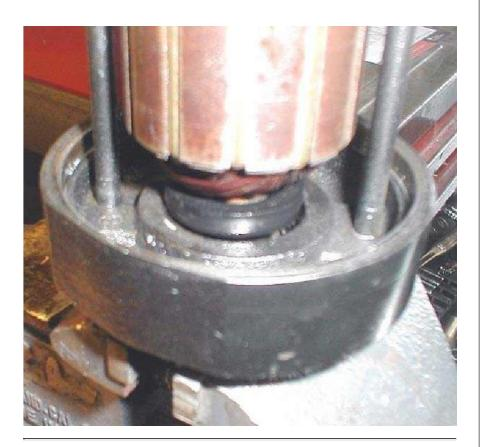
The Harley 12-volt generator has a seal in the housing that bolts to the engine case. This seal has popped out due to pressure inside the gearcase from a sumped engine.
