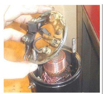
The brush plate should have enough wire to slip on after the frame and end-bell are assembled. Otherwise you may have to remove the wire or assemble the frame to the end-bell with the brush plate in place. See next step for getting the brushes over the armature. Remember the little slot in the plate and the pin in the frame have to line up.
