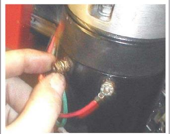
For this setup that uses a Franks Electric regulator you can hook the field and armature wires up now. Check your notes and you do have the original instructions on file don't you? Don't trust the color on these wires. Different regulators have different colors. Note the little internal tooth star lockwashers that insure good electrical contact. The hardware store is your friend. Spend time with your friends.
