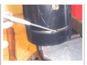
Note the little pin in the frame and the hole in the gear side end bell. It can only go together one way.
