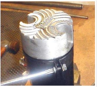
Now you can tighten the brush cover. This on is eye-balled so it points down when the generator is installed. This area was were the oil was coming out.
