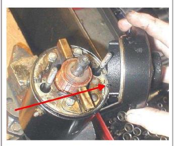
Note that same little pin in the frame picks up a slot in the end bell. It can only go together one way.
