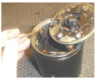
Look carefully at the little paper spacer under the square head of the field terminal. If the terminal was torqued too hard this thin paper gets cut and the field gets shorted to the armature and the generator has no output. There are some plastic spacers around. Anything including the plastic from a milk bottle is better then nothing. If you tighten the terminal up carefully you can insure the corner of the square head is not cutting through the spacer.
