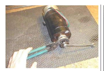
It's scary putting channel locks on a gear but that's the only way I have been able to do it all these years. Nut is conventional right-hand thread.
