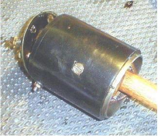
It's usually easier to put the brush plate on after the frame is installed. This plate was too snug to pop out so the handle of the mallet was used to gently tap it free. You can leave the wire attached but don't get too rude with it. I also was using paper towels to dry off any oil on the parts.
