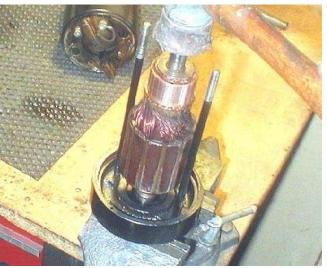
Tap the armature in with a small rubber mallet. The vise is opened up and gently tightened on the protruding rings of the end bell. You aren't supposed to use sandpaper to shine up the copper commutator because the grit gets stuck in the soft copper and then grinds up the brushes prematurely.
