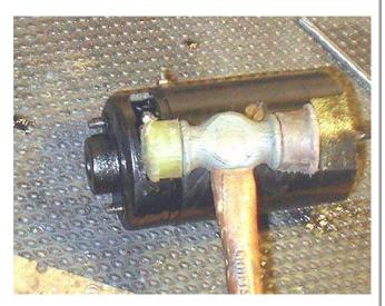
Gently tap end bell off by lightly tapping under the cutouts with a small rubber mallet. Alternate tapping on both sides to insure nothing gets bent.
