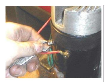
Even non meth-amphetamine addicts can strip these 10-32 brass nuts. I turn the wrench like this or use a nut-driver.
