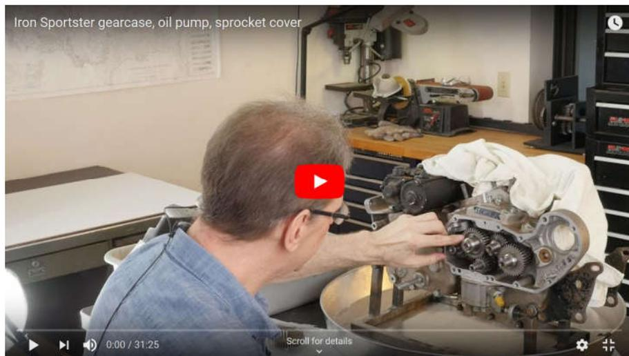
Getting the gearcase, or cam cover off is easy. Timing the cams and setting up end-play is harder. (Click for video.)
