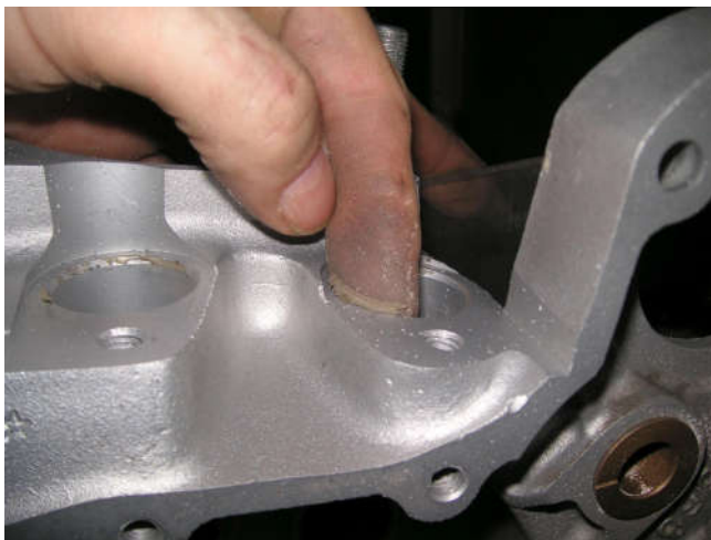
More silicone that the bead blast gun could not cut through.
