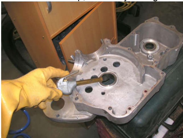
More air to get the water out. The bead blaster will blow off water, but you don't want the beads getting moist.
