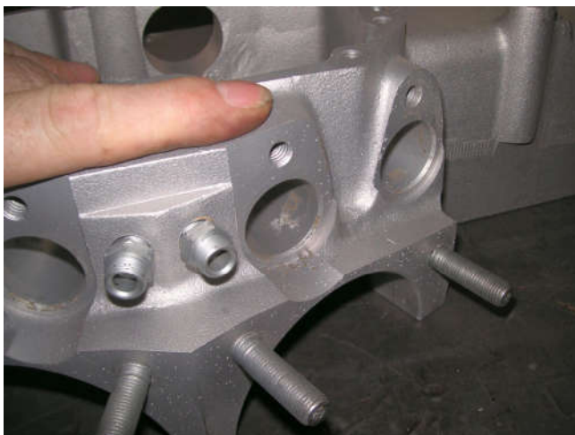
The lifter bores had a thin coating of silicone that did not wash or blow off, even with the brake cleaner.
