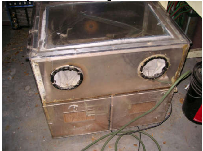
My home-made bead blast cabinet slides under the sink in the garage.
