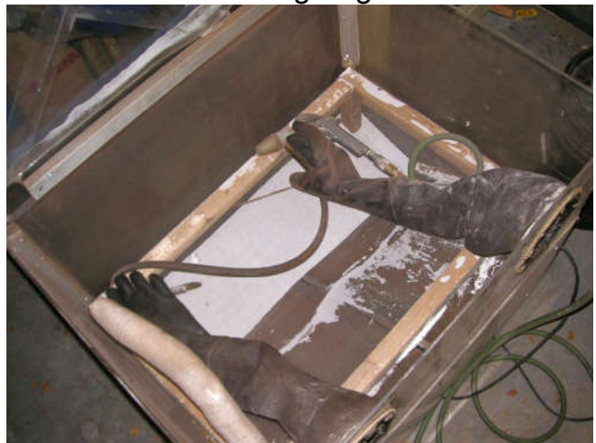
A wood frame with window screen supports the parts. Gun and gloves were from Summit Air 30 years ago.
