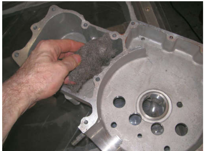
Steel wool cleans up the gasket surfaces or any sealer remaining.
