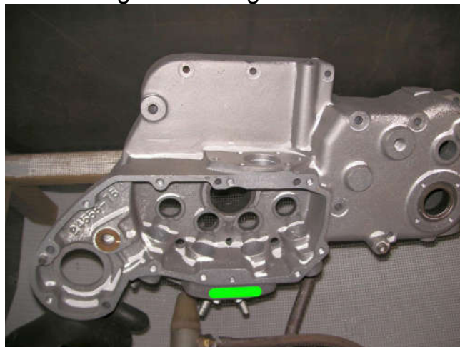
Just a little blasting and the case looks good, but the gasket surfaces need more.
