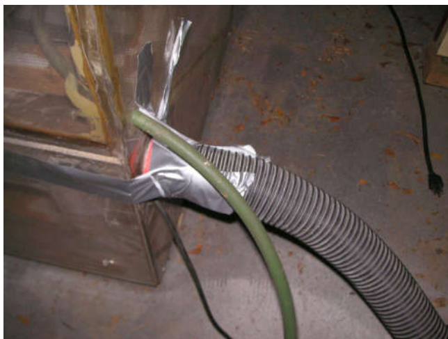
A shop vac hooks to the cabinet to compensate for the blast air coming in. The vac inside the cabinet can't keep up.
