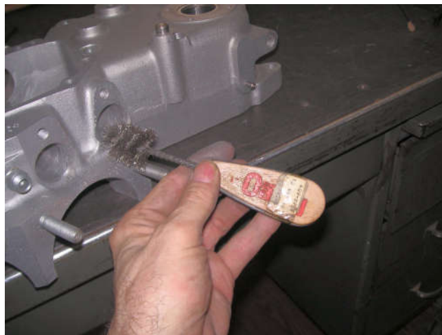
This wire brush fits the lifter bores and scrubbed out the silicone residue.
