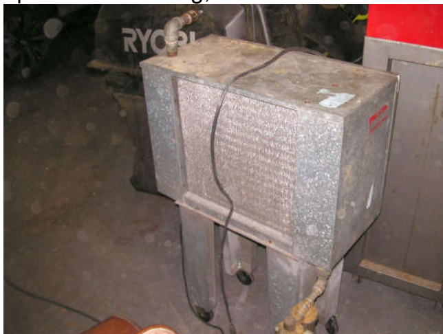
A air cooler gets the water out of the air, so the blaster does not mottle the case.
