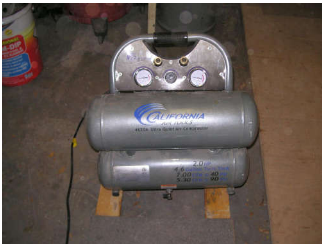
This 2-HP quiet air compressor can keep up with the blasting, with a small nozzle.
