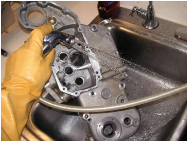
Hot water and the spray head gives some force to wash the engine case.
