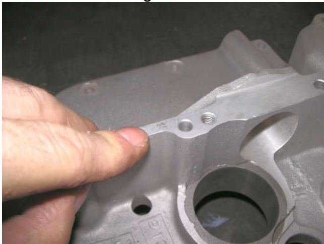
Some dirt on a gasket surface for the cam cover.
