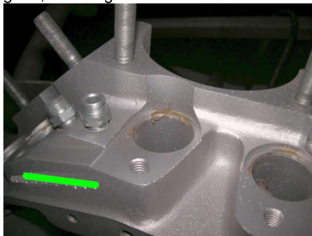
A previous owner used silicone, trying to seal the valve lifter blocks. This caused no end of grief.
