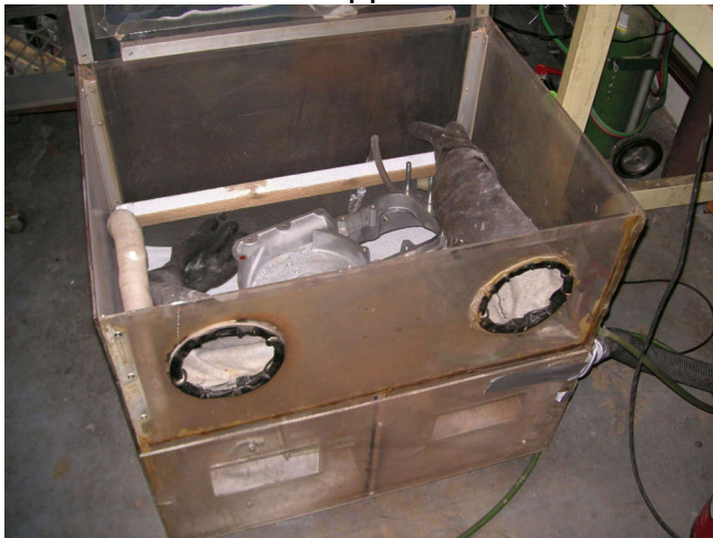
My home-made bead blaster just fits a case half. I use #10 fine glass beads.
