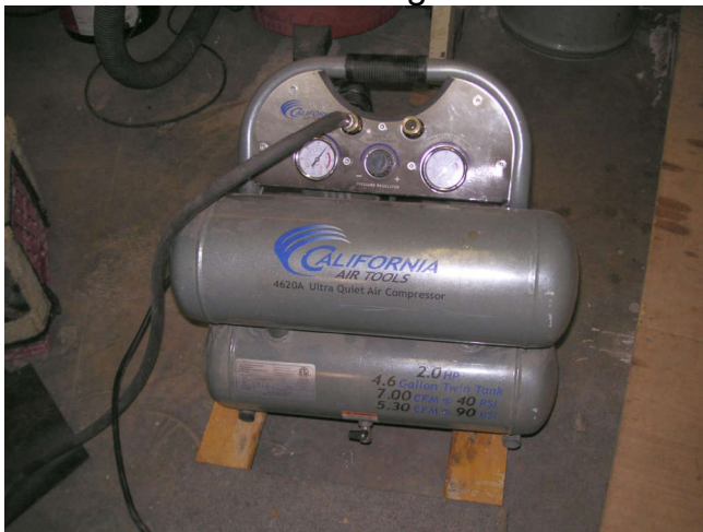
A 2-HP compressor just barely keeps up the air pressure. This one is quieter than some of the cheapest compressors.
