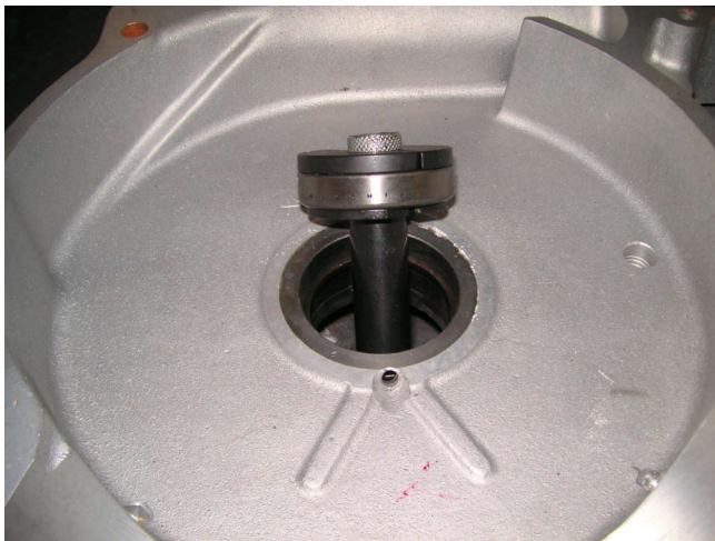
The inside race comes out like this. Support the case at the steel insert.
