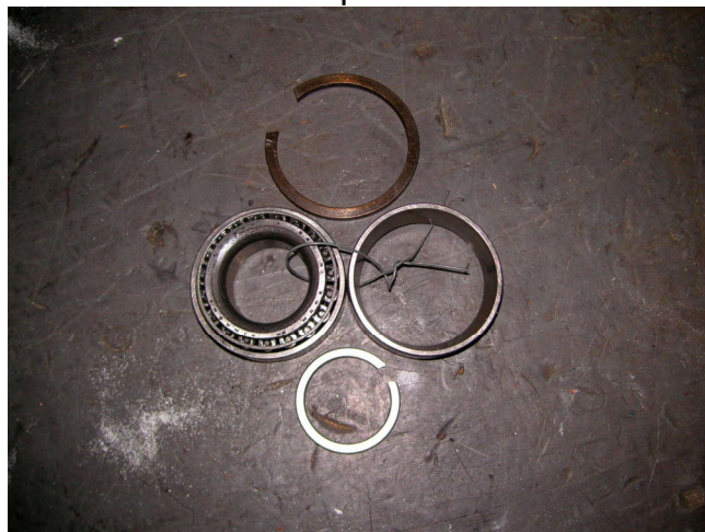
The 1977-1985 Timken race. Note the inner spacer at bottom, don't leave it out.
