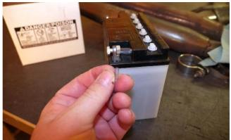
The perfect tube length to wedge in behind the nut to keep it in place.
