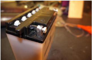
Here is the plus terminal with a section of vent tube serving to keep the nut in place.
