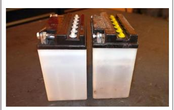
The Yuasa battery on the right has much less space behind the terminals. This means I have to keep the nut in with the vent tube placed long-ways, instead of tucked behind. It took a few tries to cut the perfect length, but it works OK. You can see the plates and acid levels seem the same. I forgot to weight them-- sorry.
