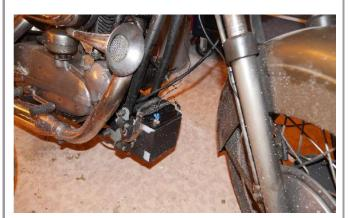
The new battery installed. I did not bench charge it, but I can top it off here before I take the bike out. I unhooked the ground just in case I have a leak somewhere.
