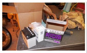
The \$27.44 battery came with acid. It was double-packed like this. I got it from an outfit called 1000Bulbs off Amazon. One thing to check is to make sure the plus and minus terminals are on the same side for the two batteries. They make this size with the terminals reversed, as I have found out the hard way. 12N7-4A is not the same as 12N7-4B.
