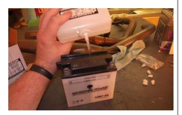
No sink setup yet in Florida, so I just was careful to not spill a drop. Be careful to not squeeze too hard or you blow the tube off the bottle and acid sprays everywhere.
