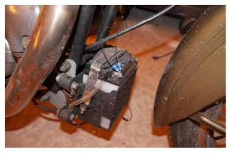
Here is the old battery. It is mounted in the XLCH box, using the normal rubber mounts. I made some brackets that tie into the front engine mount bolts to mount the box. This bike also has an experiment with 22ga Teflon wiring. It can carry the current but Teflon is too gummy for automotive wiring and can get cut.
