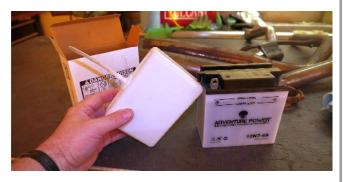
This is how much acid was left, a nice margin. You do not fill up low batteries with acid. Used distilled water. Water is what boiled off and water is what you add.
