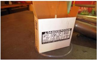
I slip the acid bottle back into its box, it just seems safer to have some cardboard to absorb any acid. The vent tube at the bottom I did not use, other than to make back-wedges for the nuts. I reused the vent tube already on the bike.
