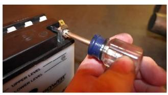
I set up the ground terminal with a spade lug. This is the nice thing about bikes without electric start. There are no high-current connections. A spade lug takes 25 amps so it is plenty.
