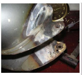
I despise fumbling with spacer washers to mount a gas tank, so I dialed in the spacers and brazed them on the front tabs of the gas tank.
