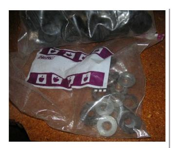
Some of those funky washers that support the rubber grommets on late-model fuel tanks, and some isolation mounts in a bag above that.
