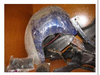
Here is the the headlamp shroud for the XLCR setup, a sissybar you can barely see, and the XLCR seat. When Kenny Puccio built the 1980 show bike, he cut off the fender mount tabs on the rear of the frame, so I am not sure I can make this stuff work.
