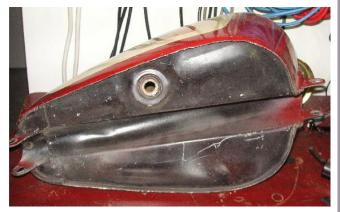
Here is the underside of the tank, you can see it has the earlier tabs to mount it.
