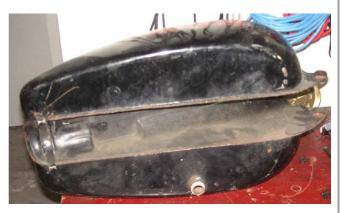
Here is the underside of the FX tank, the rear mount used a spring and rubber bushing setup.
