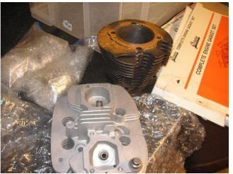
Now we get to the Thunderheads. One cylinder got wet and had surface rust, thankfully not in the bore. You can just make out the used pistons in the baggie on the left.
