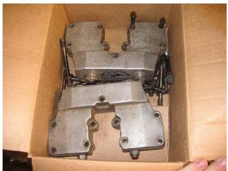
Here are the Thunderhead rocker boxes and head bolts. You use the factory Sportster rocker hardware, but cut and re-weld the arms to account for the smaller angle between the valves.
