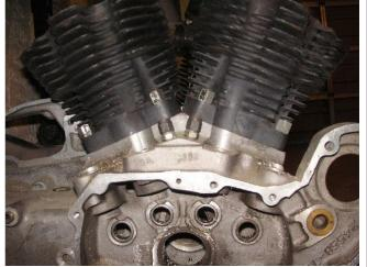
The serial number on this engine ends in "J0" so that would make this a 1980 motor. The date stamp under the front cam gear has 79 on it, so that makes sense.
