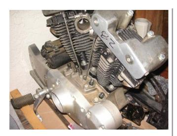
The fact that the engine has the later model integrated electric start makes it a 1981 or later. The big 82 on the rocker box is a subtle clue.
