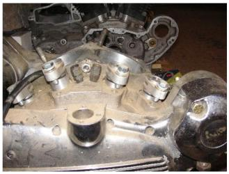
The serial number ends in "H3" so this should be a 1973. That is great, it means the tranny is stronger since there is no speedo drive down there. The missing cylinder studs worry me, but this might be a keeper to fill in the gap between my 1962 Sporty and my 1977.
