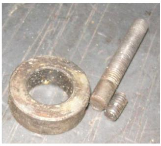
This is a little treasure to remind me when I broke the chain on my 1962. The chain wiped out the sprocket cover and broke a chunk of the case. I get it all repaired and take the bike out and it still feels sketchy and I hear the chain scraping the guard. Sure enough, this adjuster had sheared off and the chain was loose as all get-out. It never ends.
