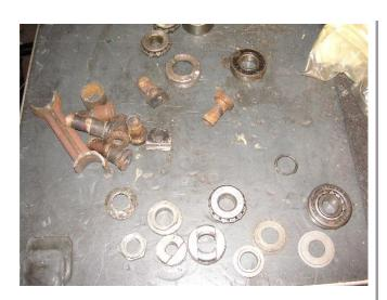
Here is some of the stuff from the can. There are frame parts, swingarm bearings, and some wheel bearings.
