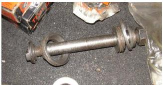
Here is a swingarm pivot. Be sure to clean up the bolt with 600 grit and lube it when you put it in the frame. I had once seize up on my 1979 bobber and took all the tricks int eh book, slide hammer, ox-acetylene torch, and in impact wrench to get it out.
