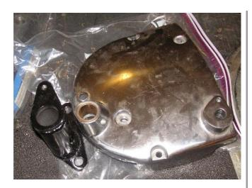
I pulled this sprocket cover and mount out of the bag so you can see it clearly. That black steel part mounts behind the cover and the kick-starter shaft goes through the tube. When you do this the sprocket cover will stop ripping in half when you kick a high-compression bike like my 1980 show bike with Thunderheads.
