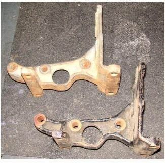
There are two types of Sportster rear motor mounts. One is steel, the other is cracked. I snag these on eBay and put them on my Sportsters. If the engine is later like a 1977 I saw off the front part of the big flat. These are later model steel, the earlier ones have a much smaller hole for the kickstarter shaft, so that it captivates the shaft and you have to either split the cases, or pull the three studs that the mount ties into.
