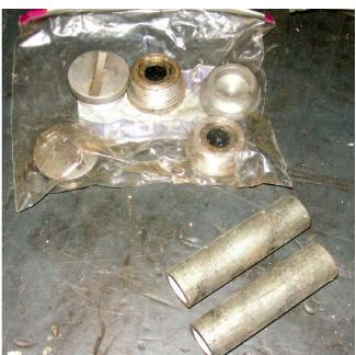
Here is a clearer shot of those primary cover oil plugs and two thick pieces of steel tubing I use to make kickstarter shaft brackets like I run on my 1977 and 1979 bobber. This gets rid of the sprocket cover.
