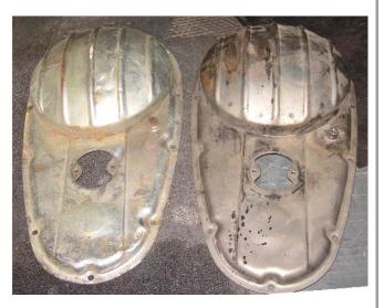
Here are two genuine Harley tin primary covers. They are two-piece. There is a separate tin cap pressed onto the cover to strengthen the dome that covers the clutch basket.
