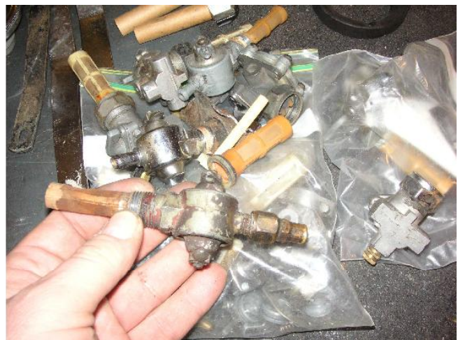
This batch of petcocks will go into the other tub, but this baby is for the K-Model as evidenced by the threaded fitting for the fuel line..
