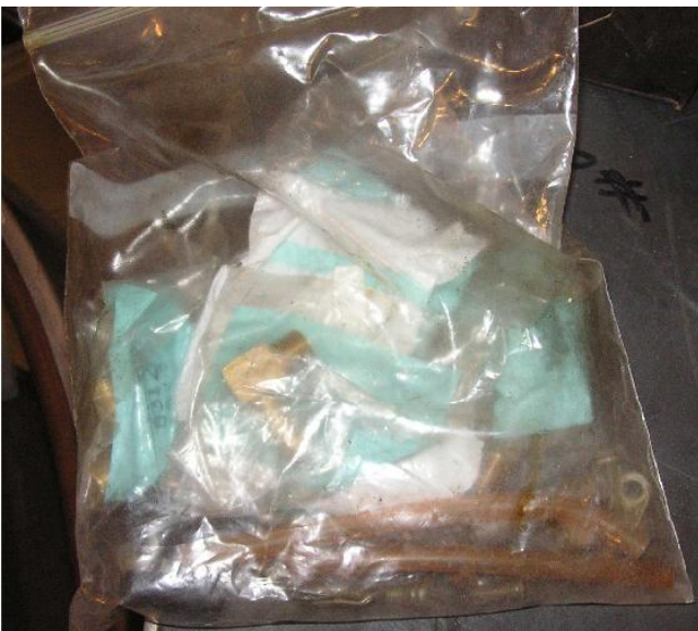
A bag of brass elbows you use to replace the black plastic leak-o-matic ones on the Keihin carb. Be sure to get 5/16 like the fuel line and don't get barbed fittings. The barbs will scrape off pieces of the hose and the chunks are certain to get into the carb. Same advice for oil lines, no barbed fittings. And that tip comes direct from racer Vance Breese .
