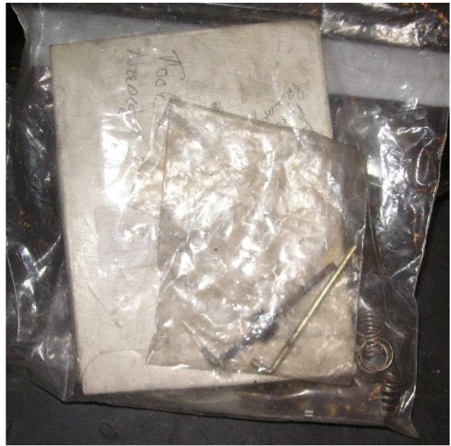
Another bag of Keihin butterfly carb parts and a rebuild kit. You need the Viton rebuild kit with this crappy gas we have today.
