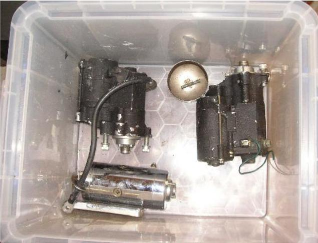
The tub had two late-model starters. Don't think these are Evo starters, the iron Sportsters went to the integrated drive starter in 1981, I know, I have an engine case that proves it. What I can't get over is how much smaller the battery is with this starter compared to that old giant H3 battery used with the 1967 to 1980 setups. There is also a chromed Prestolite starter motor in the tub.
