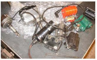
This is all the ignition stuff from that other tub. I nice magneto, and a points distributor or circuit breaker if you prefer. And seven ignition coils. The orange one has that same bracket I talked about that mounts the coil off the top motor mount.
