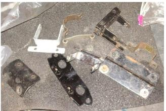
Here is a bunch of ignition coil mounts. On the far left is a home-made setup that tied to the rocker box bolts and put the coil in between the two rocker boxes on 1977 to 1984 Sportsters. Note one mount is a slot, since you can't get that rocker box bolt out with the engine in the frame.
