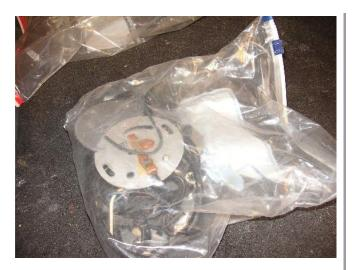
This is a baggie of factory electronic ignition pars. I used to think it was chopper and cool to have the ignition module inside the cone. Now I think maybe having it by the coil where things are less hot might be a better idea, and so then just put a sensor in the cone like the factory does after 1981.
