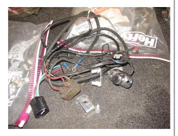
A bag of oddball wires. I figure the kill switch is ignition related, but it could go in the handlebar tub as well. That connector with the three wires is for the late-model voltage regulator.
