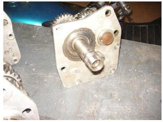
The third tranny trap door is the latter model without the boss. They stopped using the center-mount primary cover in 1966.
