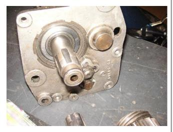
All three trannys are for 1976 and earlier bikes. This one has the threaded boss at the bottom for the primary cover bolt on dry clutch bikes with the early center-mount primary cover.
