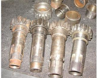
There were four clutch gears in the tub. Two on the left are early model dry clutch, then and electric start dry clutch shaft and on the far right is a wet clutch shaft.
