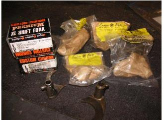
A bunch of shift forks. They come in 20 thousandths under and over, so you can set the gear spacing up. I guess they had trouble controlling the cut outs on the shifter cow paddy plate.
