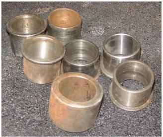
A whole mess of clutch spacer bushings, I put them in the clutch tub.
