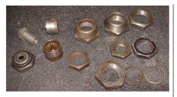
A selection of threaded stuff. A shifter plunger, some clutch nuts, and a sprocket nut or two.
