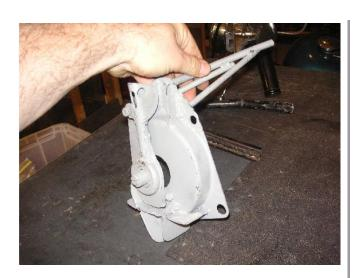
Don't laugh, here is a hack I did when I put a dry clutch in my 1977. I adapted that goofy plate that holds ht ebrake switch. I made another bracket for the kickstrarter shaft. I think this had to much pull, the hinge is not near enough to the center of the mainshaft.
