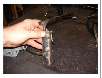
Here is another try at a clutch release mechanism for a cry clutch. Tris one worked better, but you can see that the steel bar bent so I had to weld some square stock. I cut this off the mounting plate and did a beefier design that is on my 1977 to this day.
