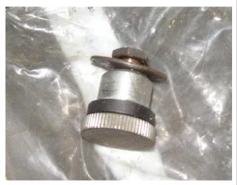
If your electric start Sportster does not have a kickstarter, but is earlier than 1981, than this is the little plug they use where the shaft goes into the primary compartment.
