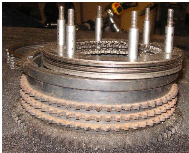
You can see some of the wet clutch steels are warped.
