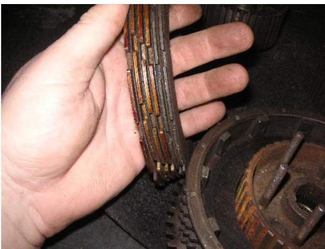
Here are some wet-clutch conversion plates for the dry clutch setup.
