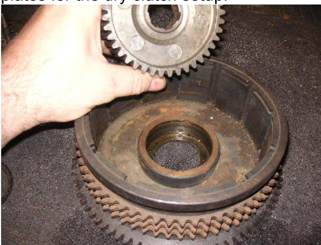
Here is a wet clutch hub and basket.
