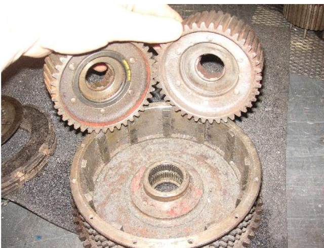
Here are the 1967 to 1970 electric start dry clutch hubs and basket.
