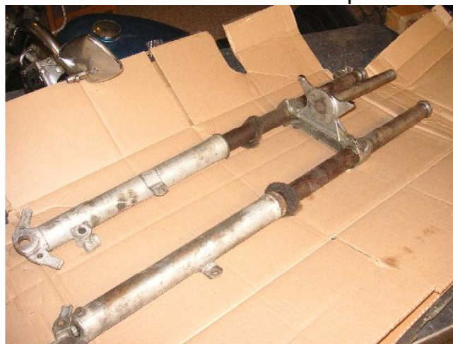
The cadmium plate is rough, but better than chrome. I hope the bushings are tight, this might be the basis of a keeper.
