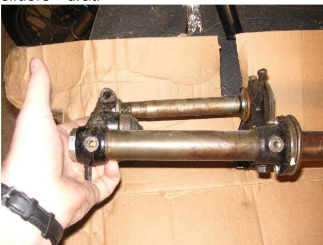
The third front end had the non-parallel setup between fork tubes and triple tree.
