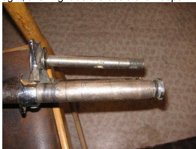
The stem on the triple tree is not parallel to the fork tubes on these early front ends.
