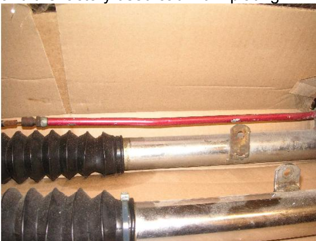
The brake cable tube got bent in the move. I can hammer this straight.
