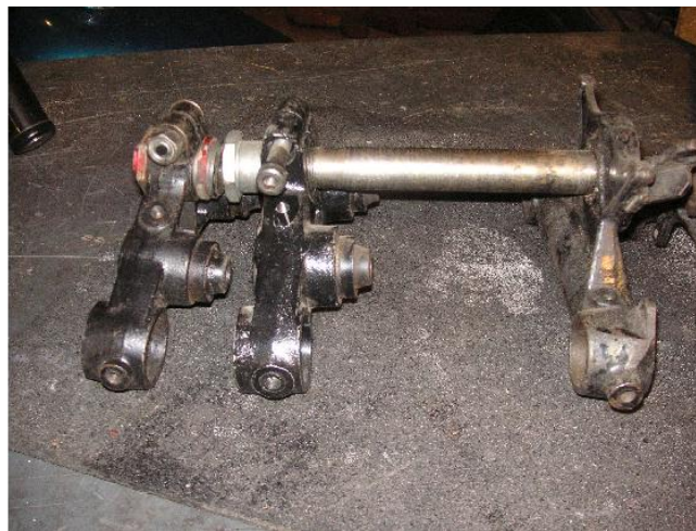
Same deal with this triple tree and clamp-- it looks more parallel. I set another triple clamp up against it, and you can see that it is different.
