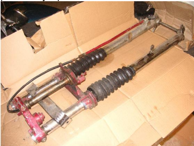
Pretty complete, the sliders are chromed, and the factory used cadmium plating.
